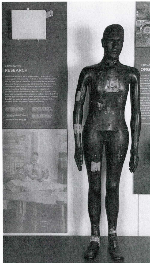
FIGURE 1. Manufactured by General Electric in the late 1940s and early 1950s, this manikin was named Chauncy by its developers at the Harvard Fatigue Laboratory in Boston and U.S. Army Research Institute for Environmental Medicine in Natick, Massachusetts. The manikin is made of copper that could be heated to maintain a constant skin temperature. They used the manikin to evaluate thermal insulating properties of military garments and headgear. (2011.0054.1) (Disclosure: This image has been spotted and cropped to emphasize the subject.) (National Museum of Health and Medicine photo/Released).
