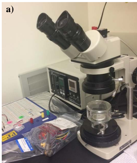
Figure 5. a) Annealing of Indium contacts b) Graphene sample with Indium contacts and gold wires attached to the contacts with epoxy.
