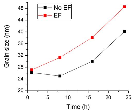
**Figure 7.** Grain size as a function of annealing time at 800°C with and without electric field (EF).
