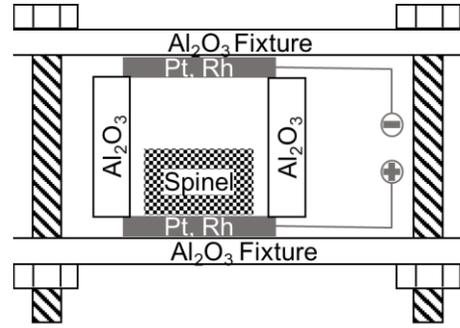
**Figure 6.** Apparatus used to polarize nano spinel pellets. Note the electrodes do not touch the samples to avoid electric current.
