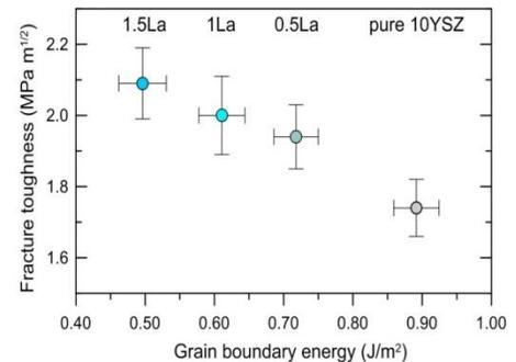
**Figure 3.** Fracture toughness as a function of grain boundary energy for La doped YSZ nanoceramics.
