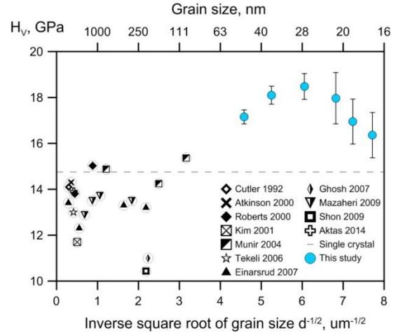
**Figure 8.** Hardness as a function of grain size for YSZ, including our data and from the literature.
