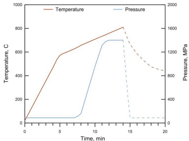
**Figure 2.** Sintering profile of HPSPS for Yttria-doped Cubic Zirconia. Starting powders were 5nm in grain size and final dense pellets were 16nm, demonstrating very limited coarsening during densification.
