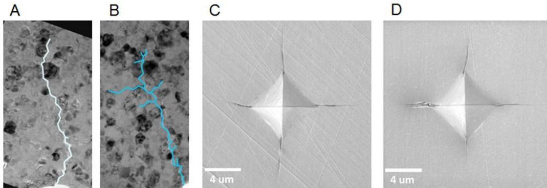
**Figure 4.** Selected images of traced cracks observed after in-situ TEM fracture tests in 10YSZ (A) and La-doped YSZ (B). Selected SEM images for the impressions on 10YSZ (C) and 1.5La8.5YSZ (D) samples left by 50gf diamond pyramid.
