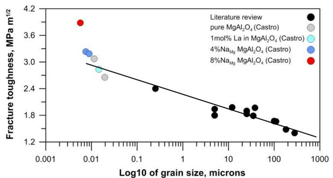
**Figure 5.** Toughness of spinel with different compositions as a function of grain size (log). Literature data marked in black circles for comparison and straight line predicts tendency.
