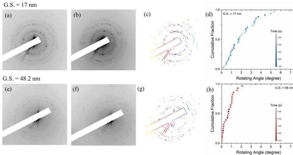
**Figure 9.** Evolution of electron diffraction patterns under applied stress. Diffraction patterns obtained during in situ TEM indentation of 17nm (a-b) and 48nm (e-f) 10YSZ samples. Tracking trajectories shown in (c) and (g) represent the corresponding crystallographic rotation. Rotation angles of diffractions spots present in the initial state and the experimental time over which they are observable (d) and (h).
