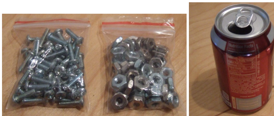
Fig. 7 Radar clutter items: (left) bag of 1/2-inch machine screws ( \times 50 ) and bag of 3/8-inch nuts ( \times 50 ), and (right) 12-oz soda can
