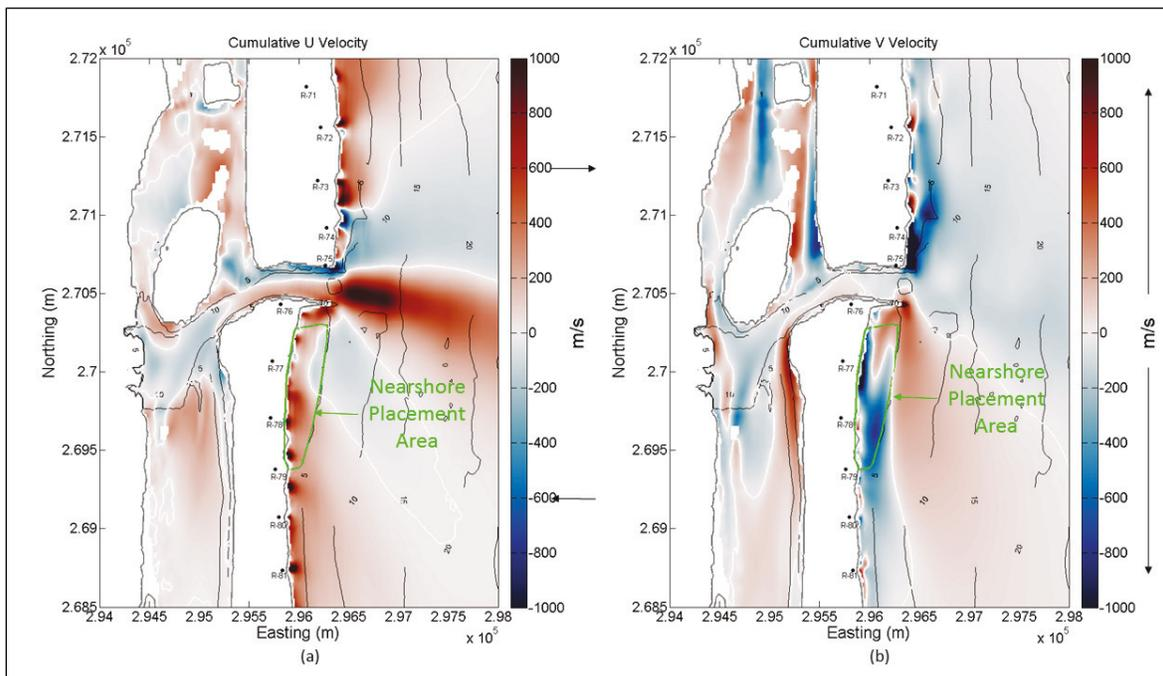
Figure 9. Cumulative velocity for year-long coupled CMS model run with regular tidal constituent amplitude forcing.
