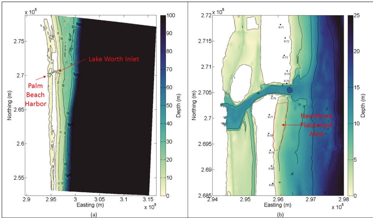
Figure 3. CMS-Wave model bathymetry (a) for the entire domain and (b) close-up view of Lake Worth Inlet area.
