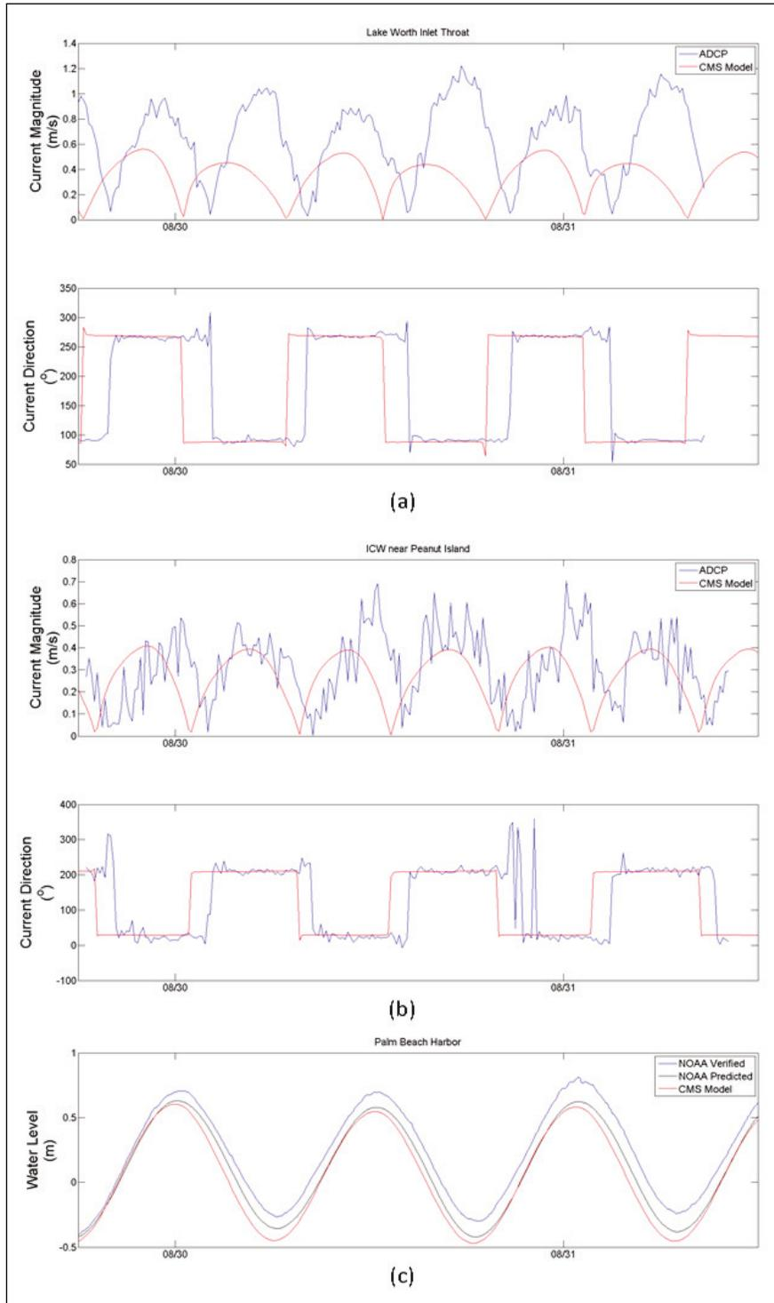
Figure 5. CMS-Flow model-computed current magnitude and current direction comparison to ADCP data (a) within the Lake Worth Inlet throat and (b) just west of Peanut Island in the ICW. Also provided is (c) NOAA-predicted, NOAA-observed, and CMS-predicted water levels at Palm Beach Harbor during neap tide conditions.
