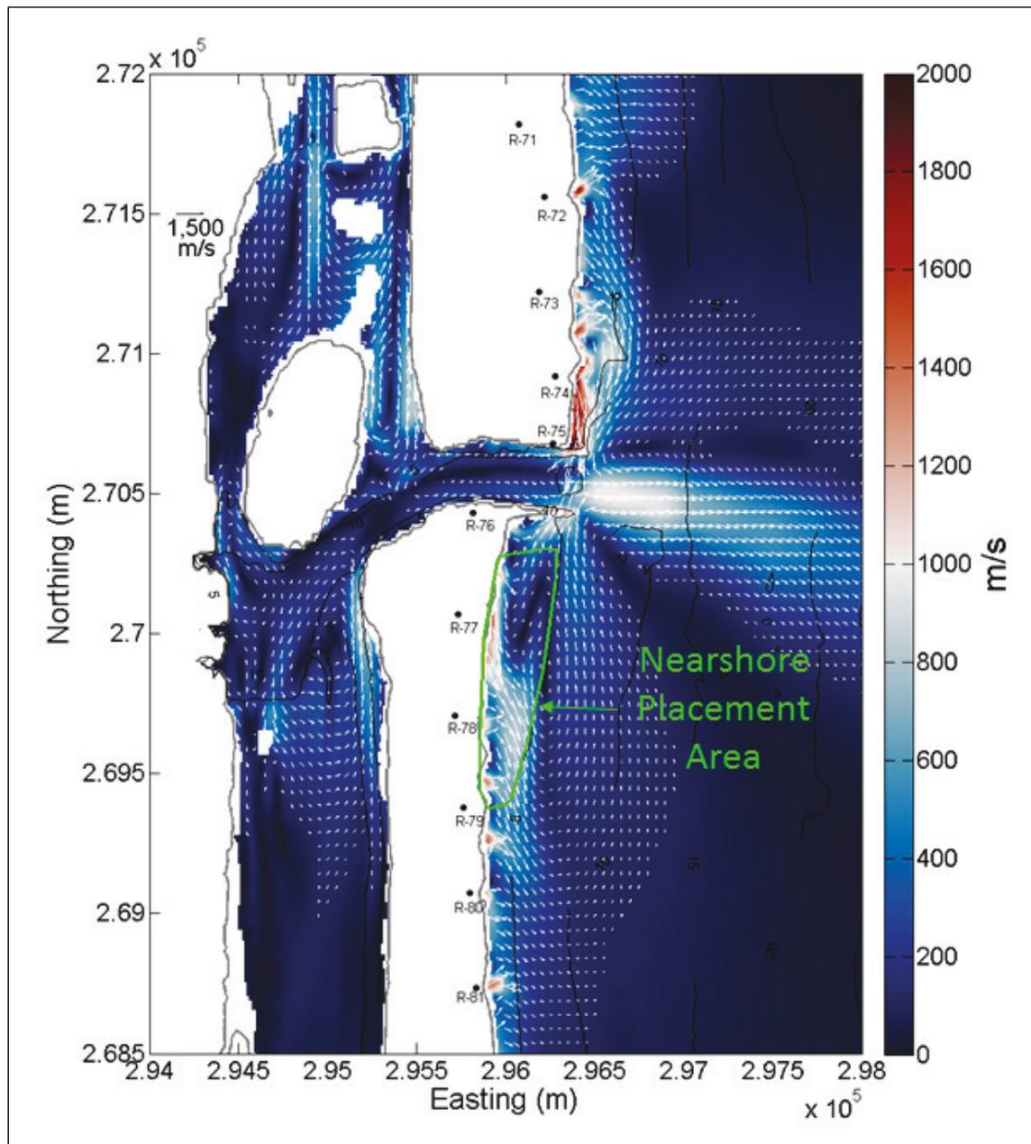
Figure 10. Velocity (a) cumulative U (east-west) component and (b) cumulative V (north-south) component, for year-long coupled CMS model run with double tidal constituent amplitude forcing.
