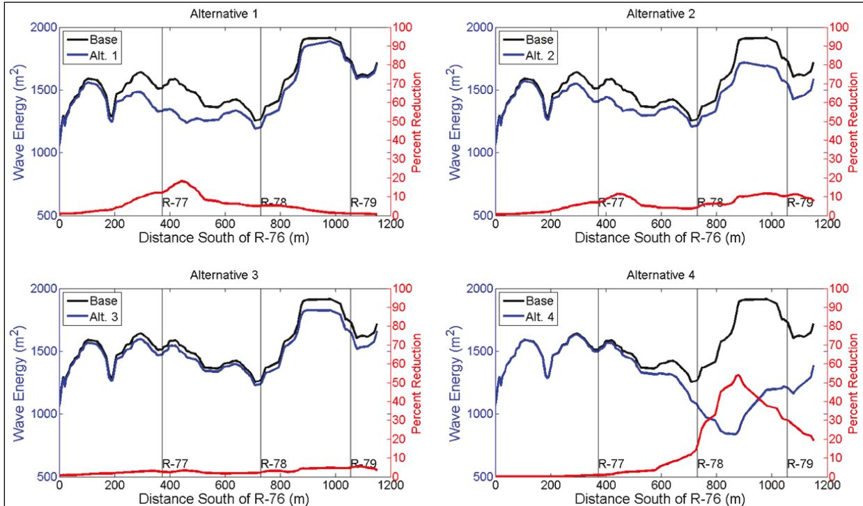
Figure 14. Wave energy percent change for Alternative 4, showing large decrease in energy in the lee of the nearshore placement area.
