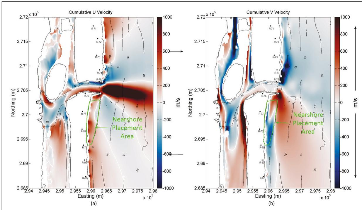
Figure 11. Cumulative velocity for year-long coupled CMS model run with double tidal constituent amplitude forcing.
