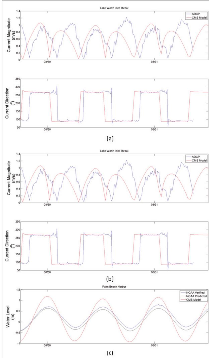
Figure 7. CMS-Flow model-computed current magnitude and current direction (with doubled amplitude tidal constituents) comparison to ADCP data (a) within the Lake Worth Inlet throat and (b) just west of Peanut Island in the ICW. Also provided is (c) NOAA-predicted, NOAA-observed, and CMS-predicted water levels at Palm Beach Harbor during neap tide conditions.
