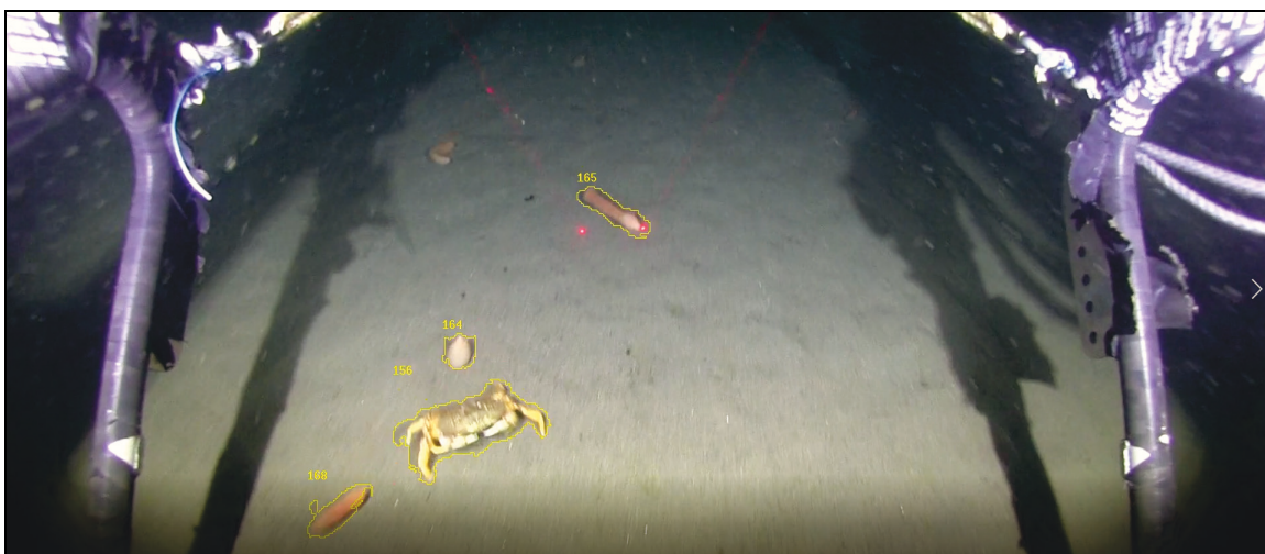
Figure 5. The Automated Visual Event Detection and Classification (AVEDAC) software tracking algorithm (yellow outline and corresponding number) detecting and tracking animals in underwater video acquired from a benthic sled (Cline et al. 2007).
