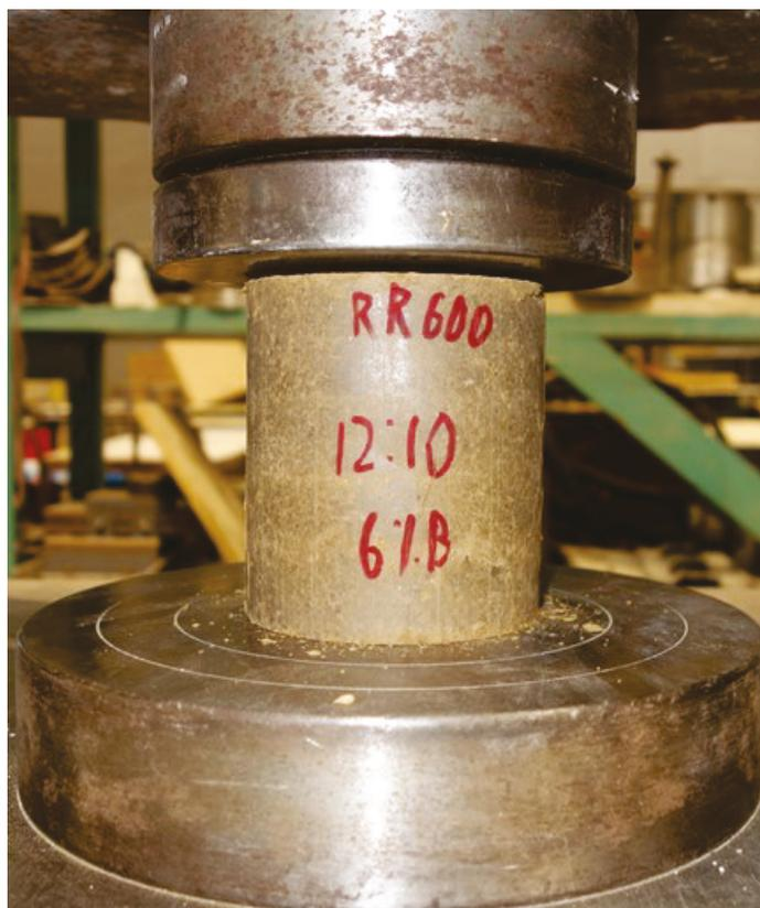
Figure 11. Two-hr UC specimen.
