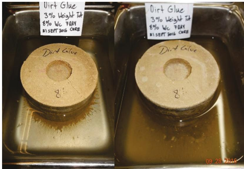
Figure 21 shows that the RR600 with reduced amount of additive stabilized silty, clayey sand specimen performed better than expected. The full additive application did not perform as well as evidenced in the pictures found in Figures 16 and 17 while exposed to partially saturated conditions over 7 days. Possible explanations can relate to mixing and curing.
