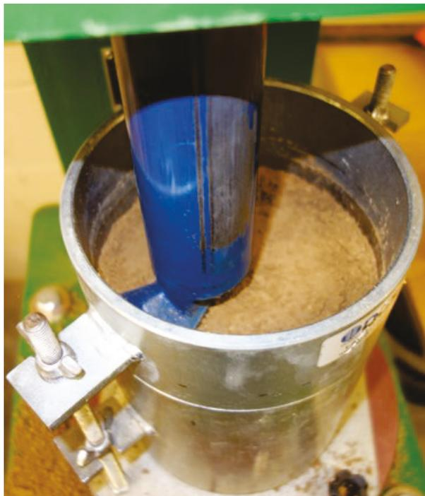
Figure 7. Humboldt H-4169 automatic mechanical soil compactor.
