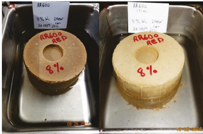
Figure 22 shows that the PLC and Class C fly ash stabilized silty, clayey sand specimen performed well while exposed to partially saturated conditions over 7 days. The images in the Figure below show the color changes and soil particle suspension.
