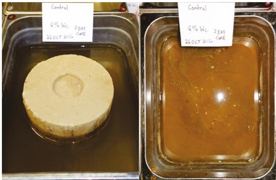
Figure 20 shows that the RR600 stabilized silty, clayey sand specimen performed very well while when exposed to partially saturated conditions over 7 days.
