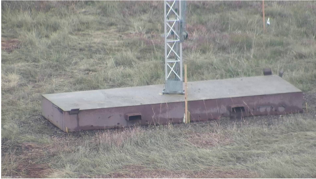
Figure 5: Portable base of a tower of the NWTC acoustic tomography array.
