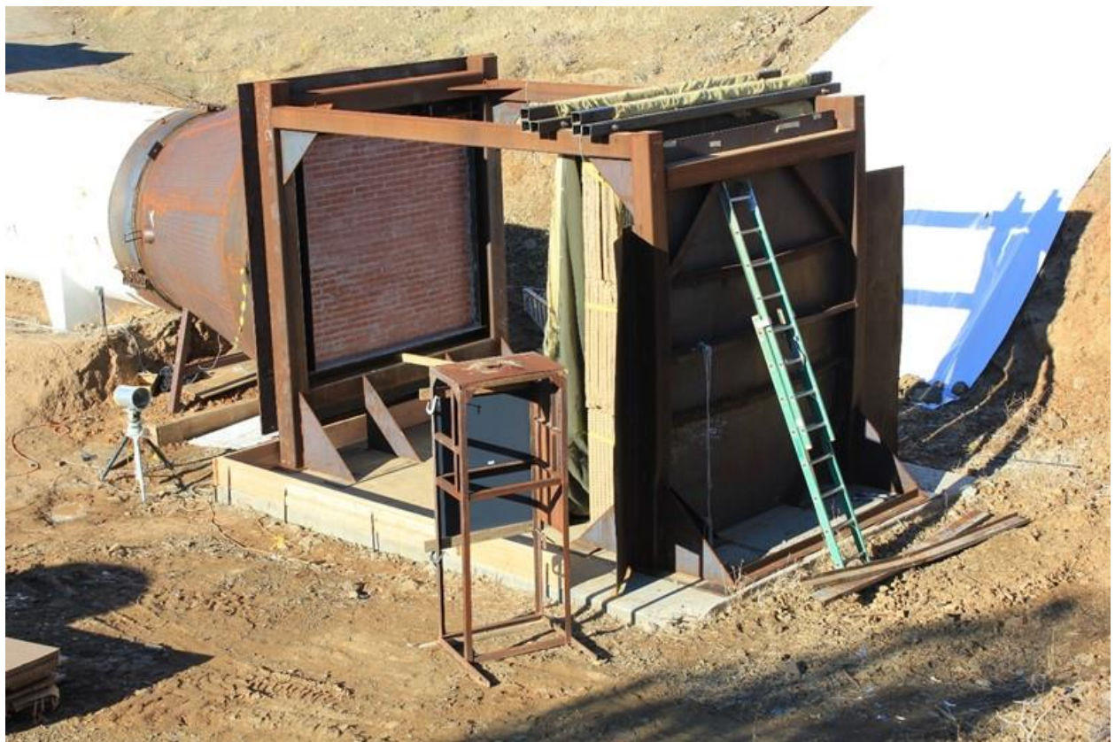
Figure 7. Shock tube with a test sample and measurement equipment in place.
