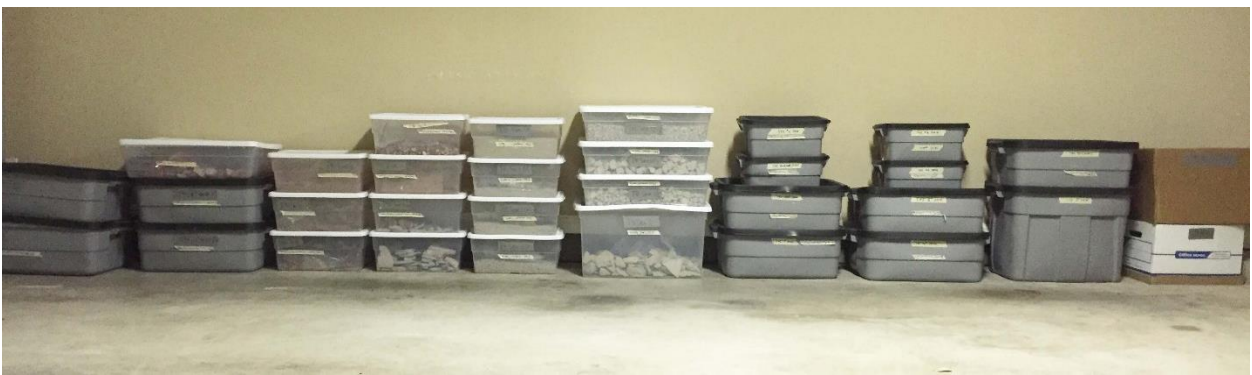
Figure 24. Fragments generated in the test series sorted into size bins through sieving.
