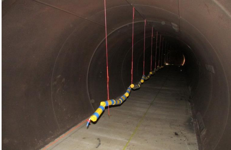
Figure 8. Photograph of the explosive driver inside the shock tube.
