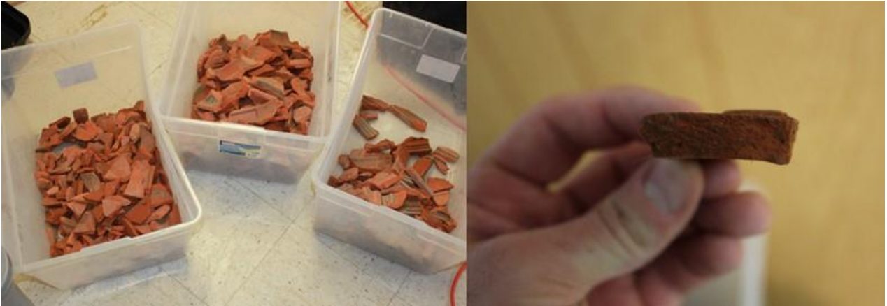
Figure 23. Photographs of clay tile roof fragments produced in Test 43.
