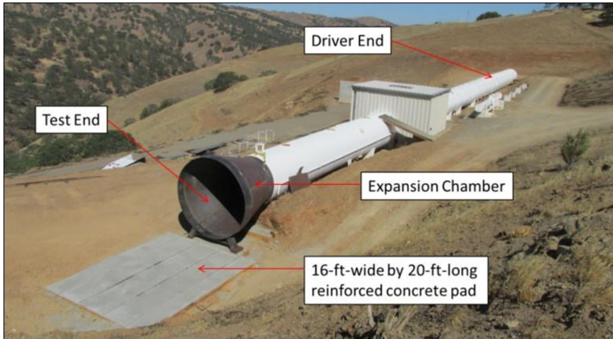
Figure 6. Shock tube used in this test series.
