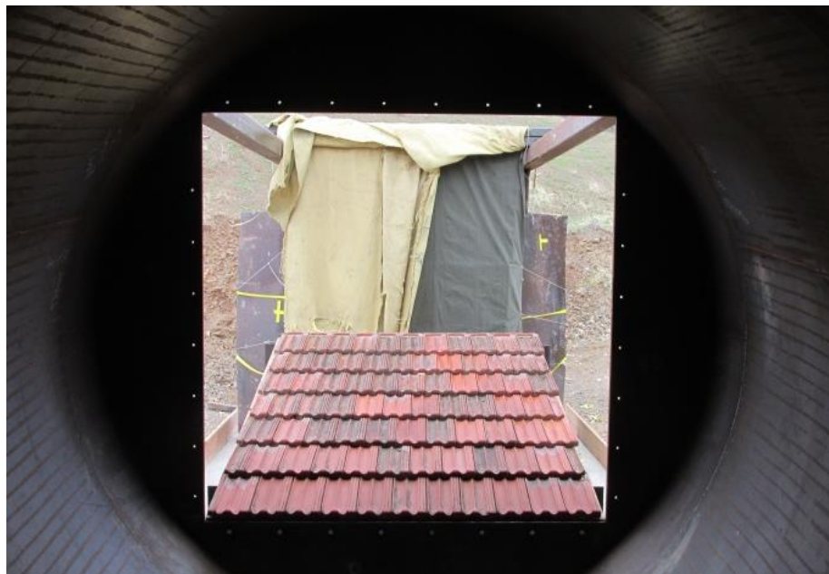
Figure 5. Pre-test views of the clay tile roof sample used in Test 43.
