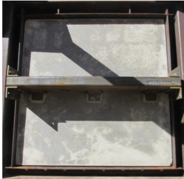
Figure 3. Rear view of the reinforced concrete spandrel panel sample used in Test 42.
