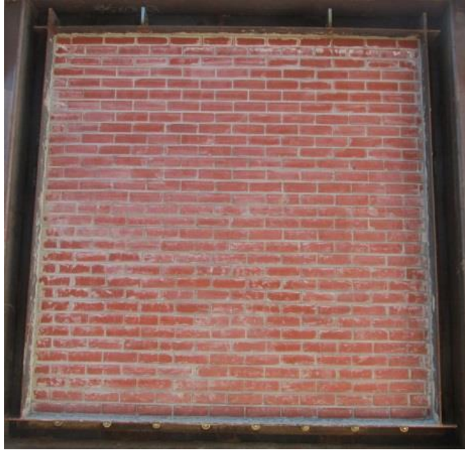
Figure 1. Rear view of the brick wall sample used in Test 40.
