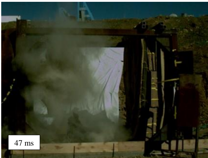
Figure 19. Later-time failure of the concrete spandrel panel in Test 42 as recorded by the overview HSV camera.
