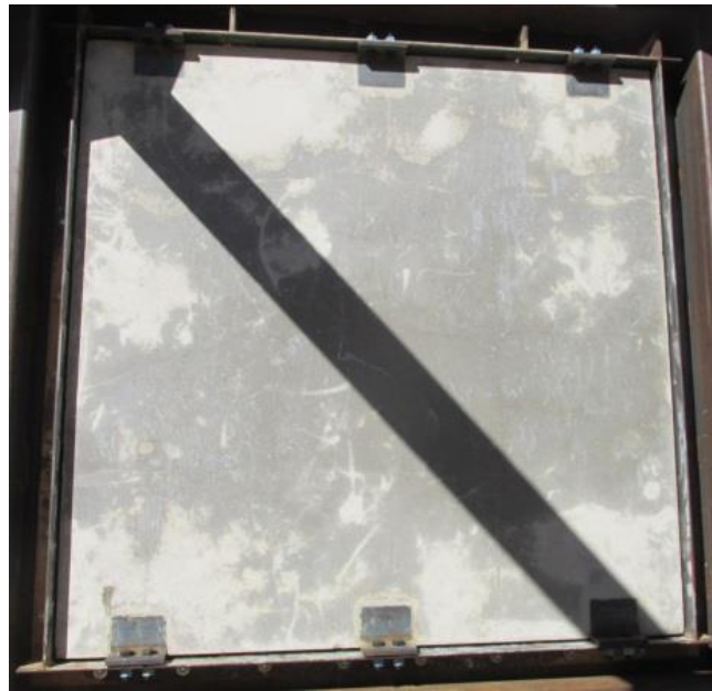
Figure 2. Rear view of the reinforced concrete structural panel sample used in Test 41.
