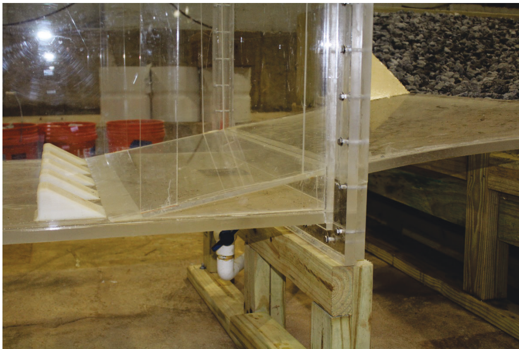
Figure 28. Fillet added in stilling basin, dry.
