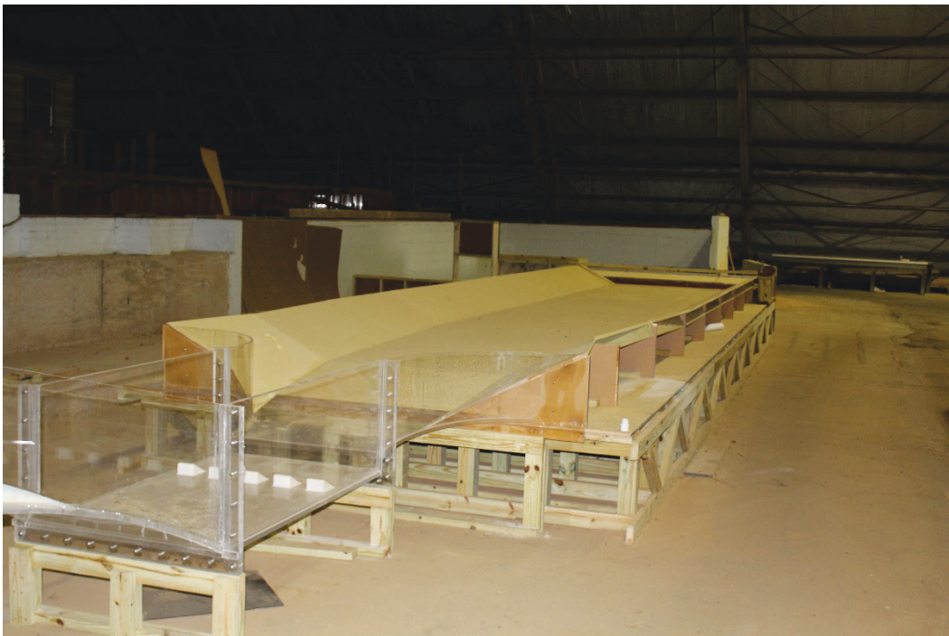
Figure 16. View looking downstream of exit channel constructed of marine grade plywood.
