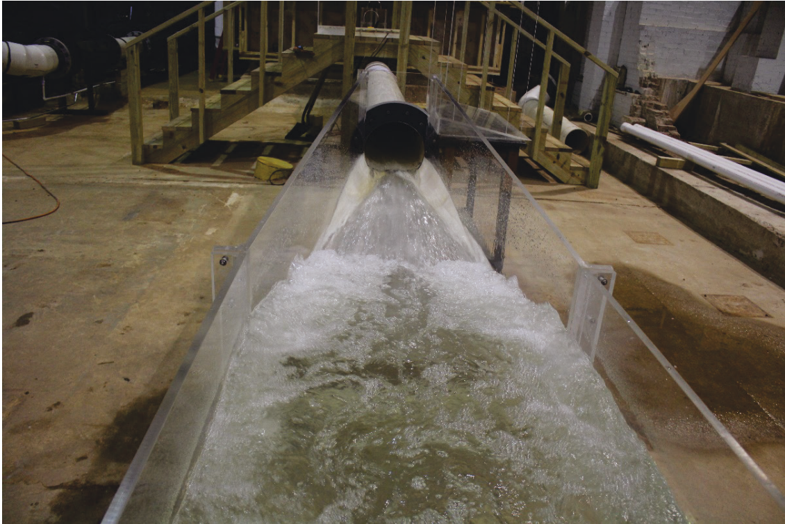
Figure 33. View looking upstream with a discharge of 1,000 cfs and the inverted V installed.
