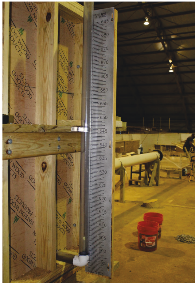
Figure 10. Elevation marker – head bay.
