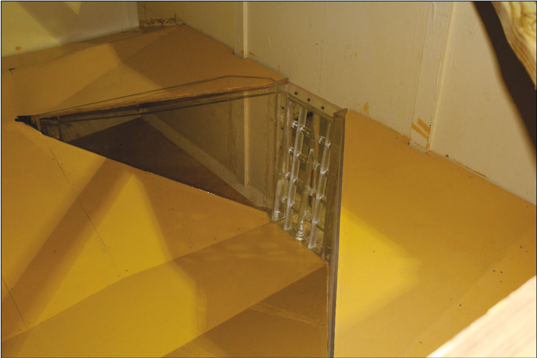
Figure 7. View looking downstream of trash rack and approach channel.
