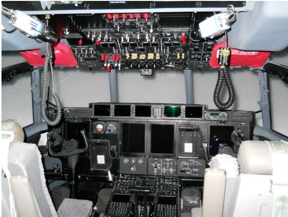
The inside of a Lockheed C-130J Super Hercules Weapons System Trainer used to provide realistic simulated flying training to J-model students. (Photo taken by 314 AW/PA; USAF Photo). 111
