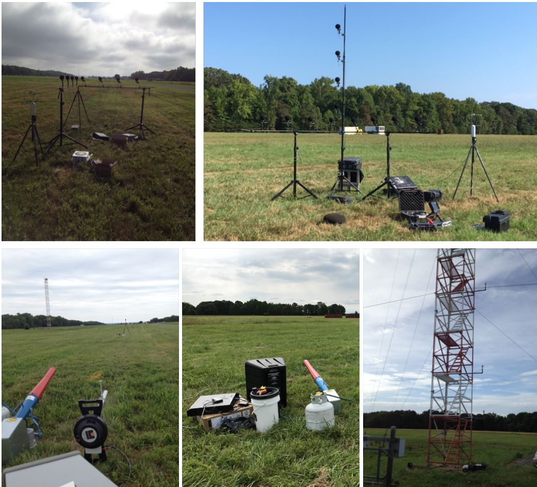
Fig. 7 Instrumentation. Upper: two-axis array (left); three-axis array and sonic anemometer (right). Lower: propane cannon and speaker (left and center); met tower with Airmars (right).
