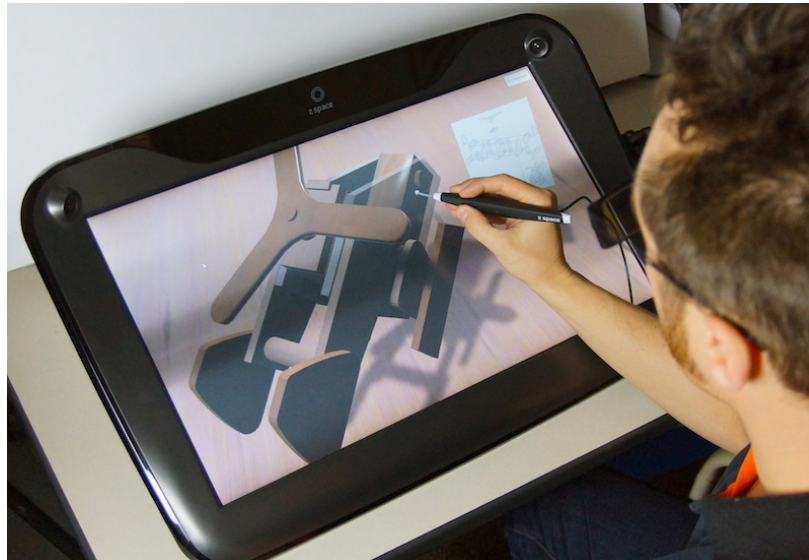
Figure 5. Non-immersive zSpace display with head tracking and unimanual stylus interaction
