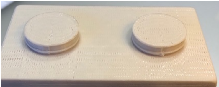
Figure 19. Connections on 3D printed parts with bumps added for easier assembly
