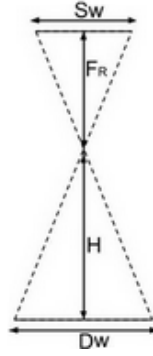
Figure 8. Parameters affecting GSD. Source: PIX4D (2017).
