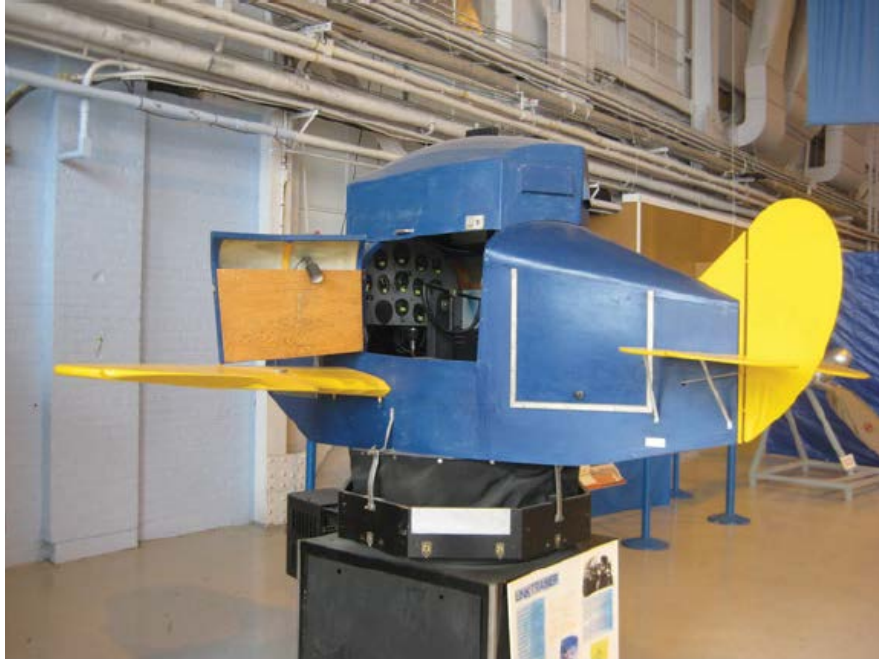
Figure 1. The “Blue Box” by Link Aviation. Source: Stanković (2016).
