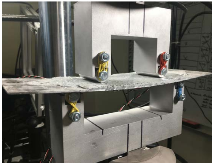
Figure 20. Experiment I: Sample G End of Testing—Before Unloading
