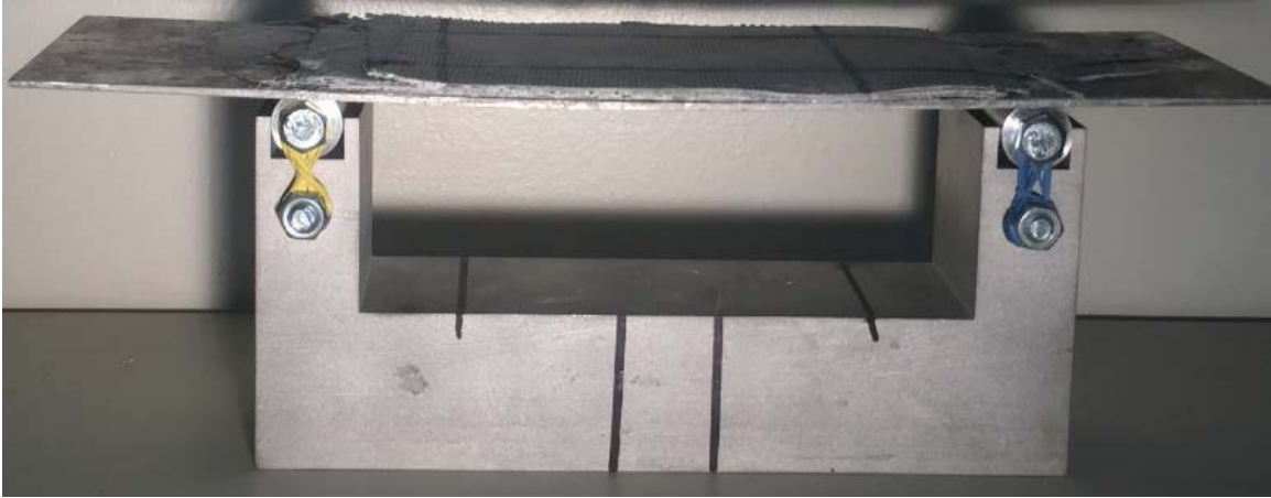
Figure 28. Experiment I: No Permanent Deformation Shown in Sample I
