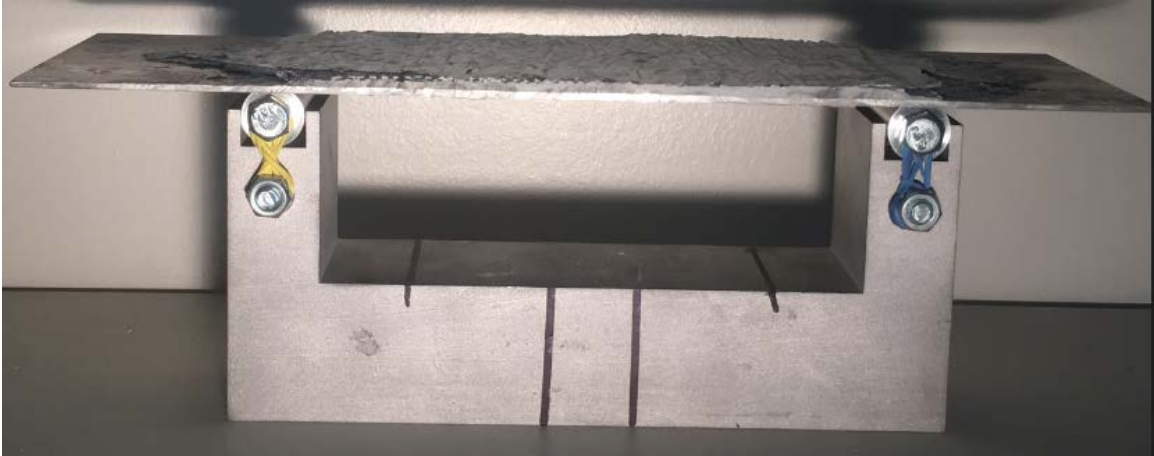
Figure 23. Experiment I: No Permanent Deformation Shown in Sample H
