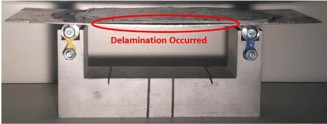
Figure 33. Experiment I: No Permanent Deformation Shown, but Delamination Occurred in Sample K
