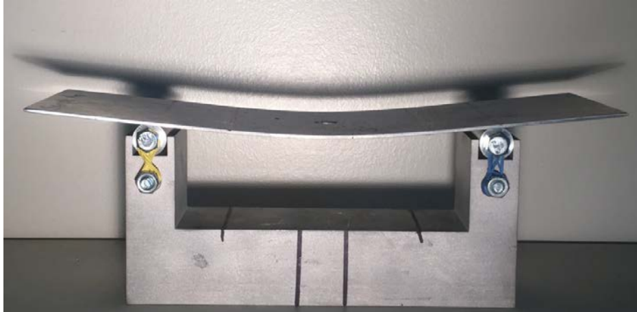
Figure 8. Experiment I: Permeant Deformation of Sample A
