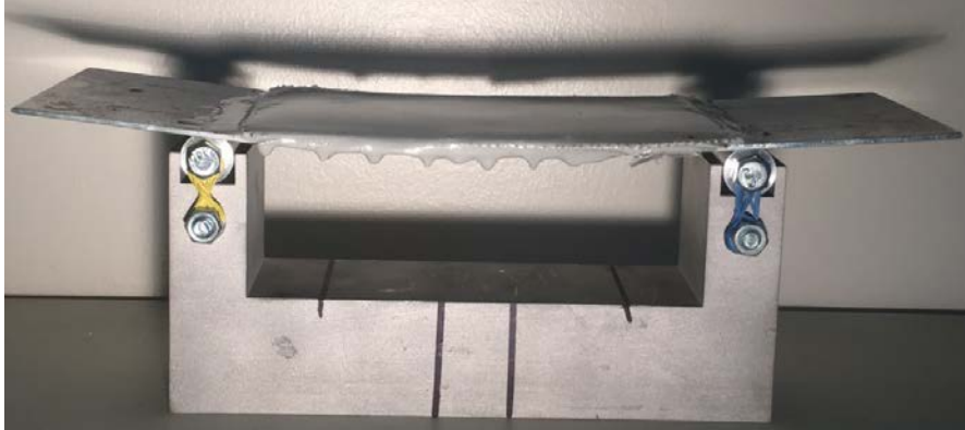
Figure 13. Experiment I: Permanent Delamination of Sample C
