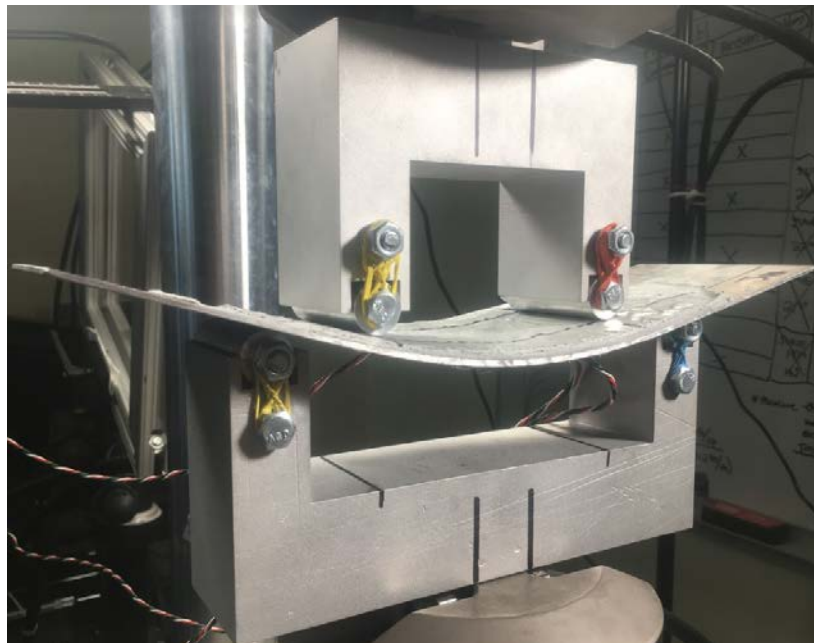
Figure 27. Experiment I: Sample J End of Testing—Before Unloading
