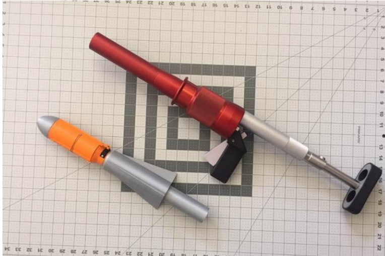
Figure 3. Projectile prototypes with parachute deployment system and stabilizer fins.
