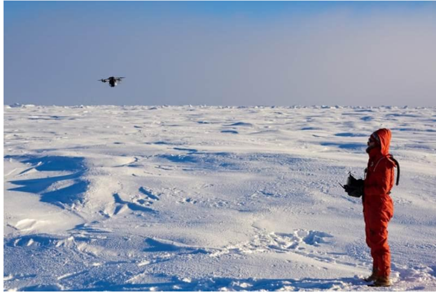
Figure 13. Dr. Peter Guest flying the InstantEye UAS with radiosonde over Arctic sea ice. (Photo by Byron Blumquist)
