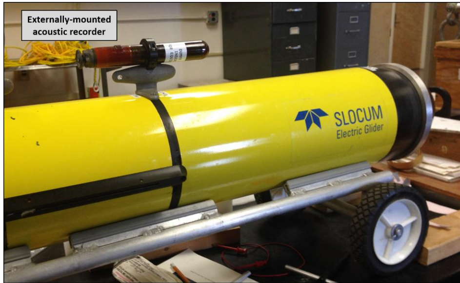
Figure 19. OC Slocum glider with externally mounted acoustic recorder
