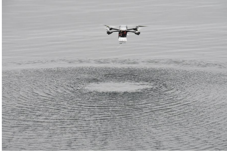
Figure 14. The InstantEye UAS/ radiosonde flying over the Pacific Ocean, generating small waves. The InstantEye is about 1 foot across and is hovering about 18 inches over the ocean surface. (Photo by Tom Murphree)
