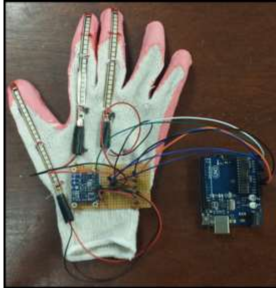
Figure 48. Fully assembled glove controller with flex sensors, IMU and Arduino Uno microcontroller.
