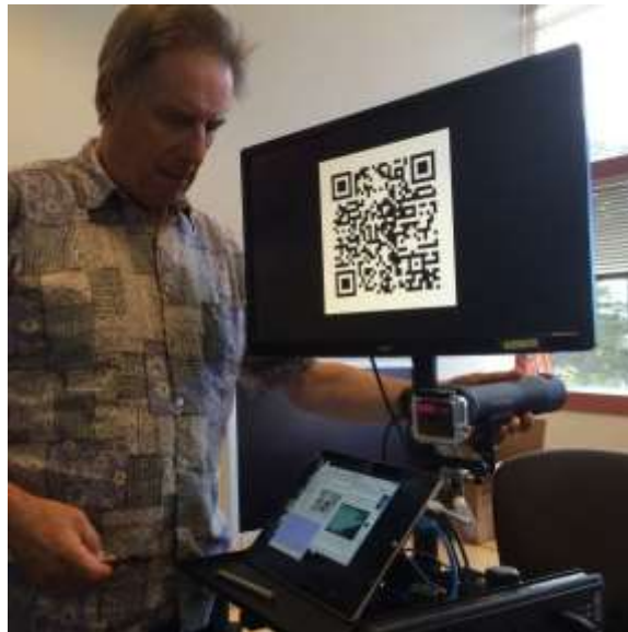
Figure 8. Mike Bailey with 20x telephoto lenses working with the GoPro Hero 4 cameras. Modifying the camera cases to hook up cabling allowed for full image throughput to our Java-based QR tactical decision aid (TDA).
