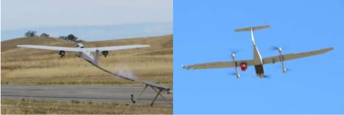
Figure 41. Catapult-launched and vertical-takeoff deployment platforms.
