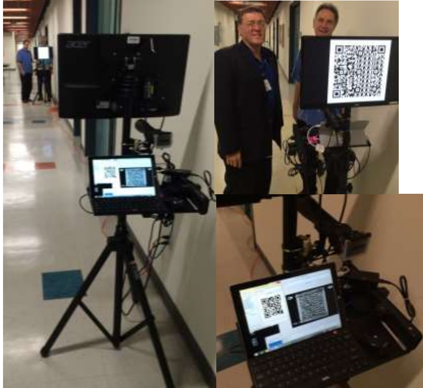
Figure 9. Test rig components include standard computer display monitor, 20x lens from Torrey Pines, GoPro4 camera with 4K resolution, Standard COTS cable connectors, Microsoft Surface3/Windows8 tablet, and NPS-written open-source Java software with live video display/interface and QR code generator, reader. Tripod mount, can ride on dolly.
