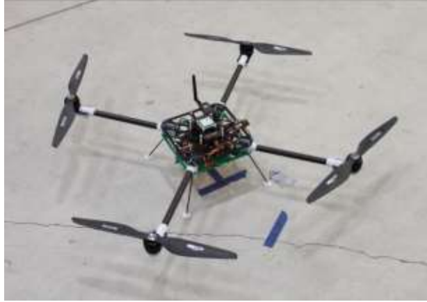
Figure 28. The "dry" prototype airframe currently undergoing flight testing in the USL motion capture (MoCap) space.
