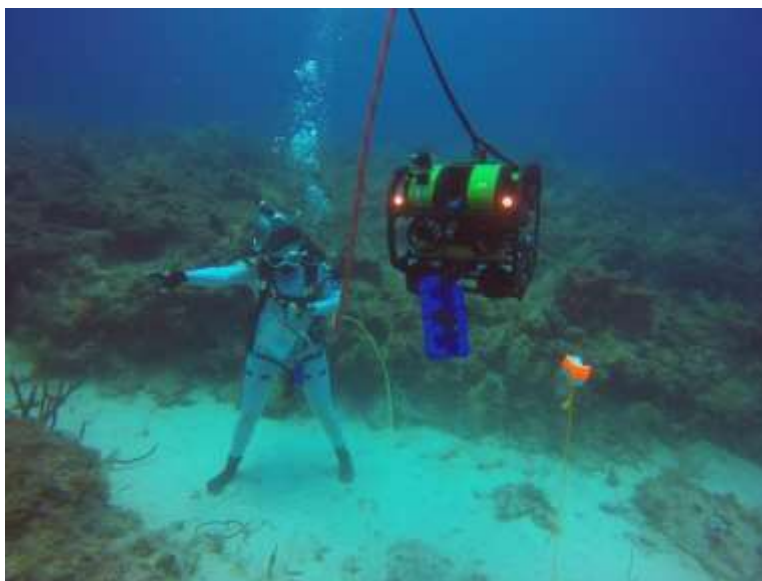
Figure 16. Semi-autonomous collaboration decreased the burden on divers during exploration tasks. ACQUAS carried samples and documented scientific tag locations.
