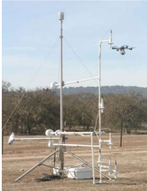
Figure 25. InstantEye/Radiosonde alongside calibrated meteorological tower.
