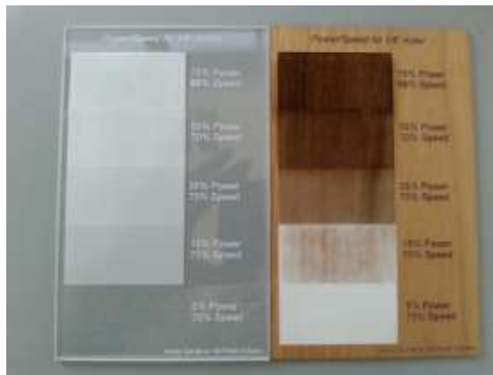
Figure 55. Laser Test Samples: Power and Speed Settings
