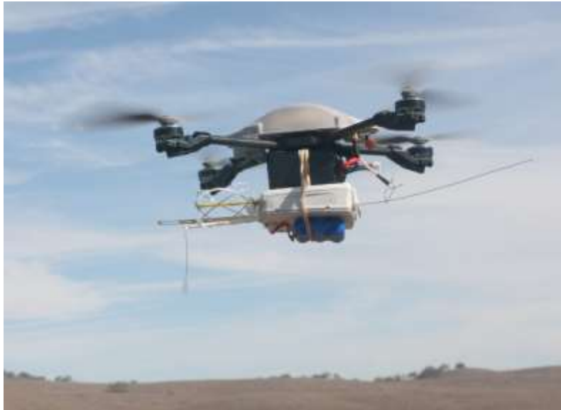
Figure 24. The InstantEye Unmanned Aerial System with radiosonde meteorological sensing system attached.
