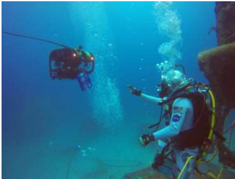
Figure 17. ACQUAS shuttles tools and gear between work sites and the Aquarius habitat, delivering science samples to an awaiting Aquanaut.
