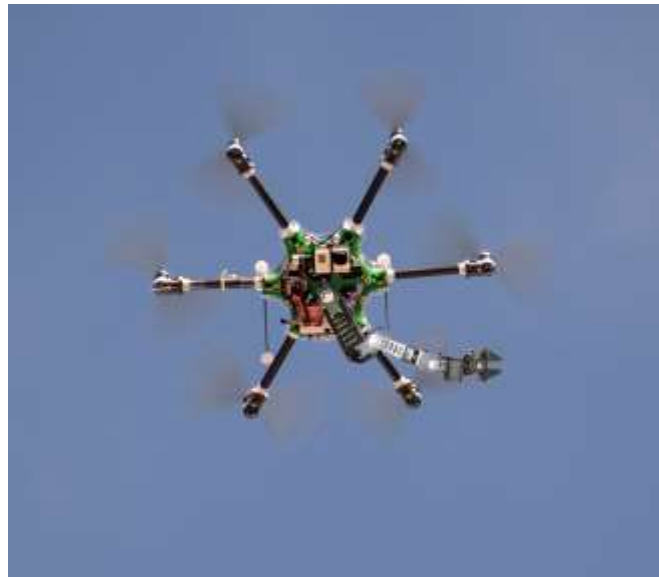
Figure 36. Artist rendering of the "Manicopter", a multicopter based robotic manipulator
