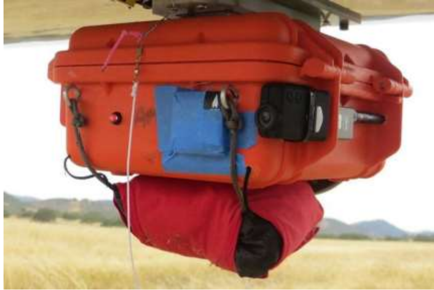
Figure 39. Snowflake aerial delivery package under the wing of UAV.
