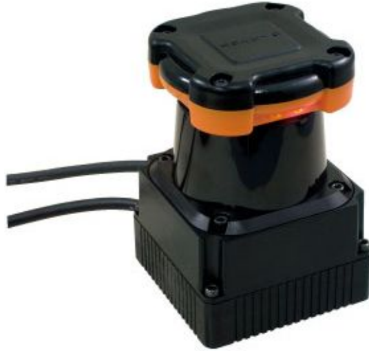
Figure 5. The Hokuyo UTM-30LX Scanning Laser Rangefinder. Source: [11].
