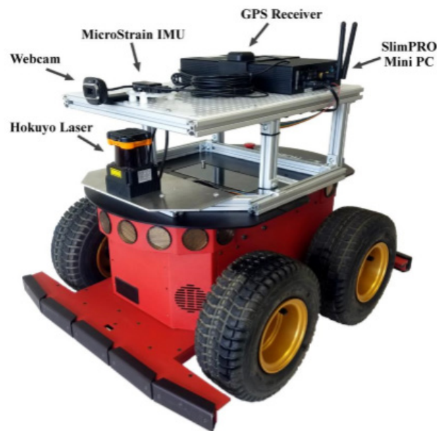
Figure 7. P3-AT with Sensor Suite as Used in Experimentation. Source: [6].
