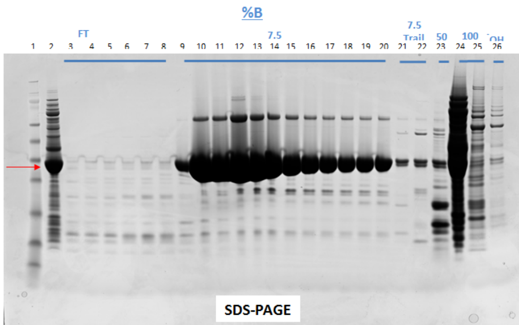
Figure 2. Purification of LdNH36 from E. coli using ion-exchange chromatography. The target protein, LdNH36, consistently runs as a doublet band with slightly different profiles on a non-reduced 4-12% BisTris gel. Electrophoresis was carried out in MES running buffer (per Thermo Fisher instructions). The gel was run at 125 Volts for 40 minutes and stained with 0.25% Coomassie Blue R-250, then destained with successive washes of 5% methanol in 7.5% acetic acid.
