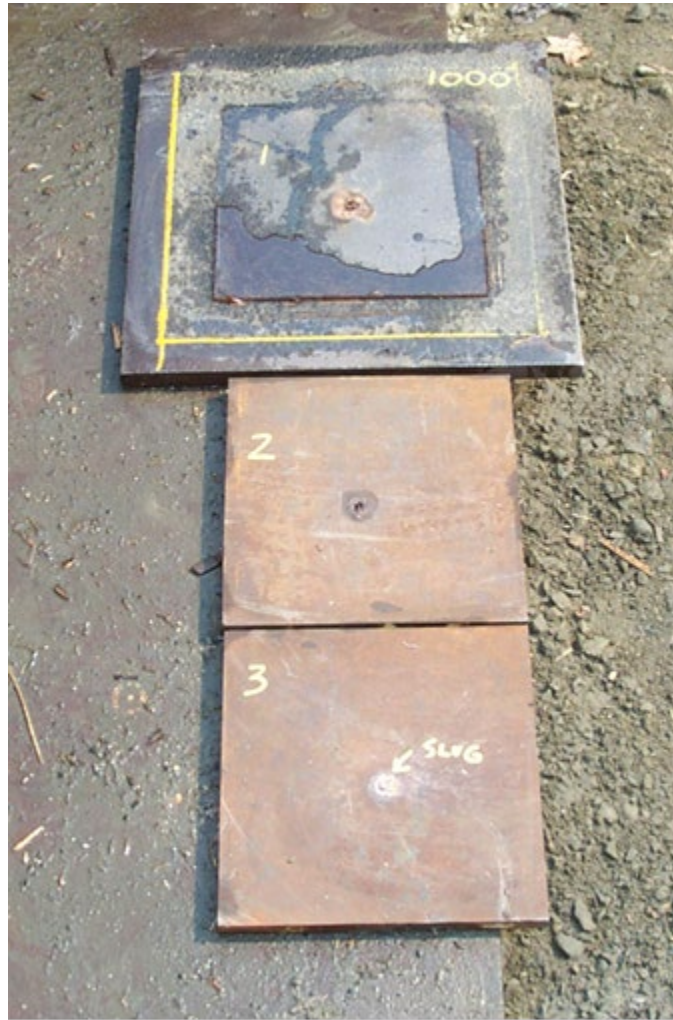
Fig. 4 Typical postexperimental debris. Debris from target with 1000 mm of water is shown. The jet stopped in witness plate No. 3.
