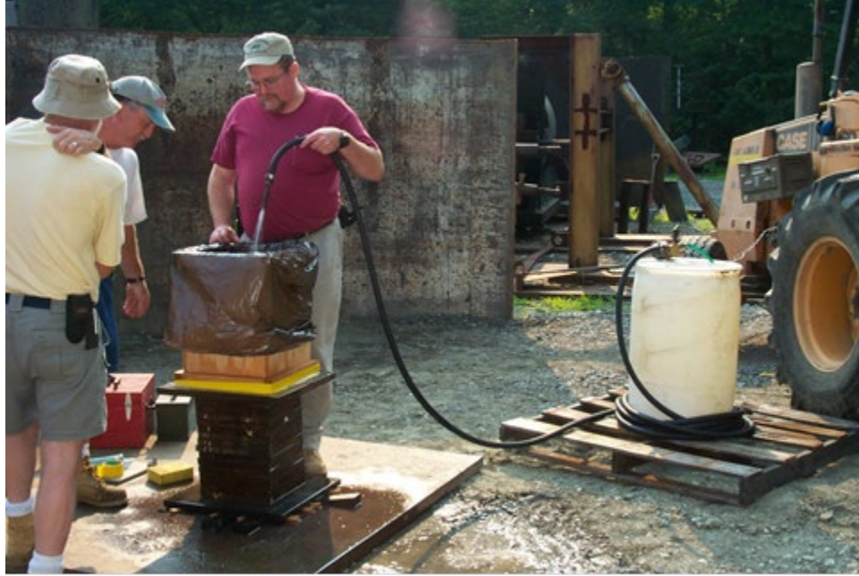
Fig. 2 Filling target with 500 mm of water
