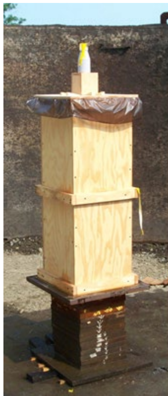
Fig. 3 Typical experimental setup. Target with 1000 mm of water is shown. The wood target assembly has a hole cut in the top so the first material impacted by the shaped charge jet is water.
