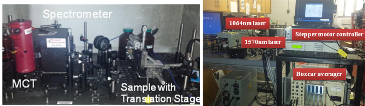
Figure 2: Picture of the eye-safe IR LIBS system (left), pump laser systems (1064nm & 1570nm), and associated control and data acquisition equipment (right).
