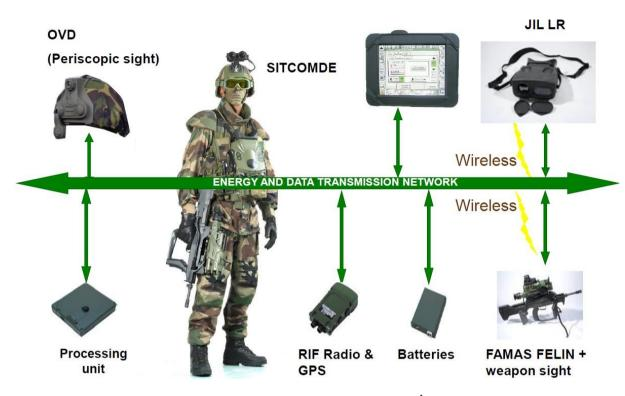
Figure 2-12: Energy and Data Transmission Network of the FÉLIN Soldier System [21].
