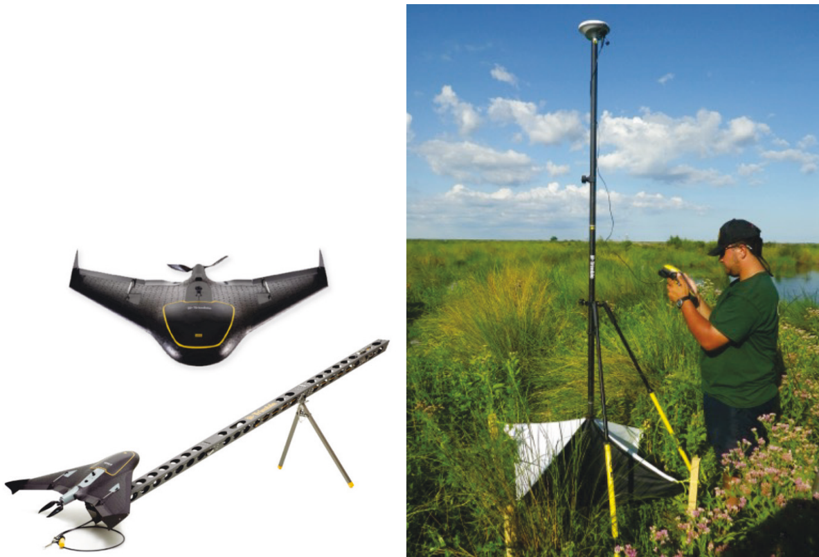
Figure 2. UX5 aerial rover (left) and surveyed ground control point (right).
