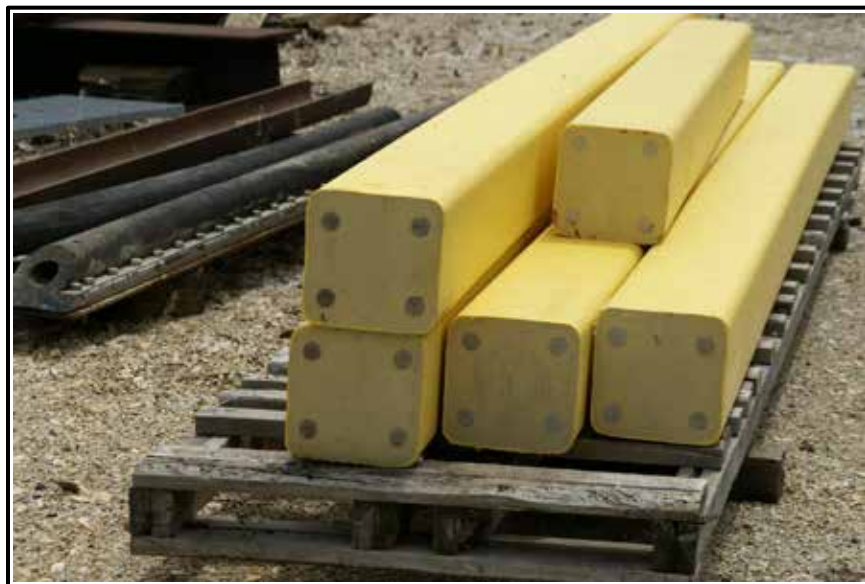
Figure 2-20. Composite rebar reinforced HDPE timbers. Note yellow color throughout the cross-section.
