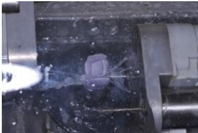
(Figure 20: milling chamber and fabrication of veneer prosthesis)
