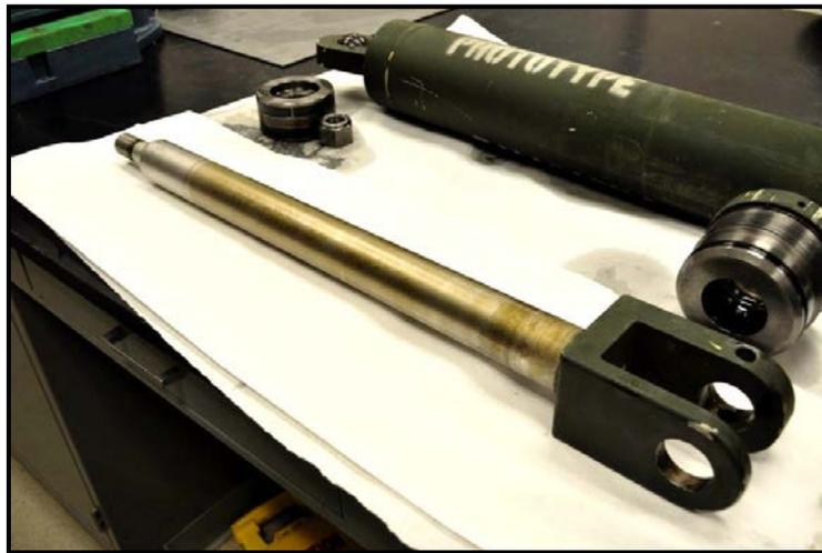
**Figure 6-9. Image of Unassembled Prototype Dem/Val Cylinder Assembly Following Two Months of Field Exposure on the M9 ACE.**
