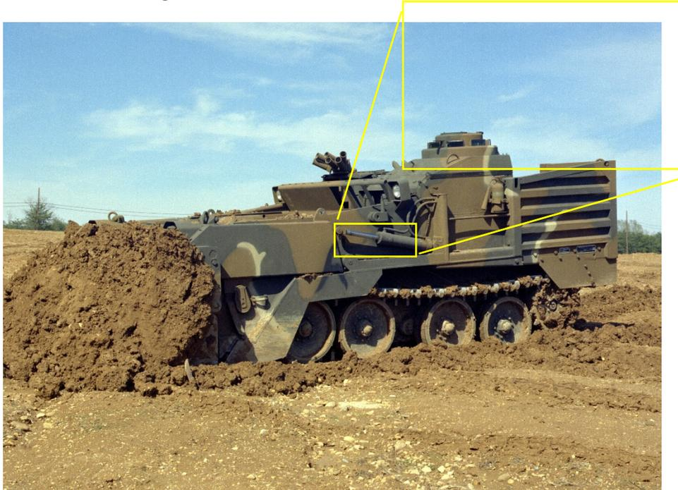
**Figure 4-6. Image of M9 ACE Vehicle with an Inset Image of the Hydraulic Cylinder Coated with EHC Plating.**
