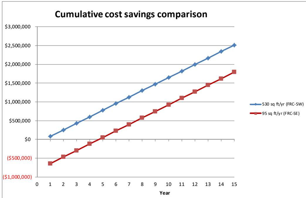
**Figure 7-2. Comparison of Cumulative Cost Savings for nCoP Implementation at a Low-volume Depot (such as FRCSE) and High-volume Depot (such as FRCSW).**
