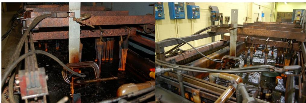
**Figure 4-8. Image of a Chrome Plating Tank Currently in Use at FRCSE.**
