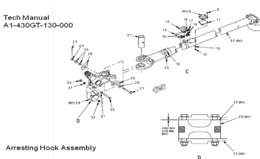
**Figure 4-3. Technical Manual Excerpt with a Detailed Schematic of the Arresting Tail Hook Assembly.**
