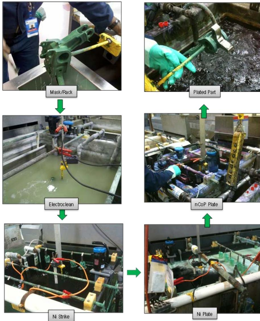
**Figure 6-2. Visual Illustration of the General Plating Process Flow.**
