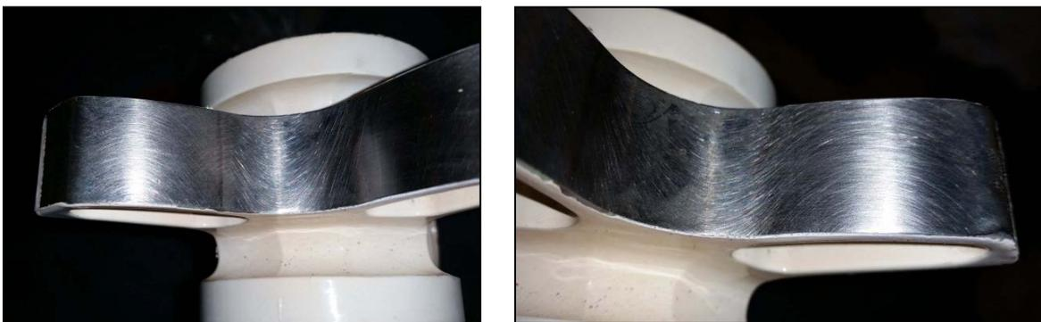
**Figure 6-4. Images of Cam Surface of nCoP plated Pivot Following 97 Arrestments.**
