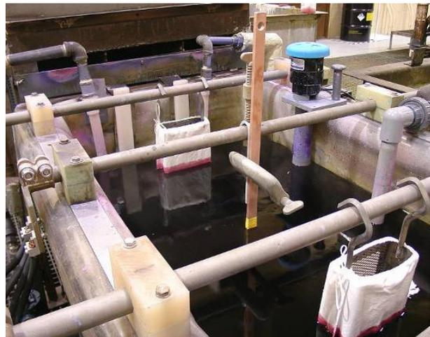
**Figure 5-2. Photograph of 300 Gallon nCoP Plating Tank at FRCSE.**
