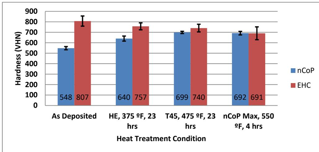
Figure 6-1. Microhardness of nCoP and EHC at Various Heat Treatment Conditions.
