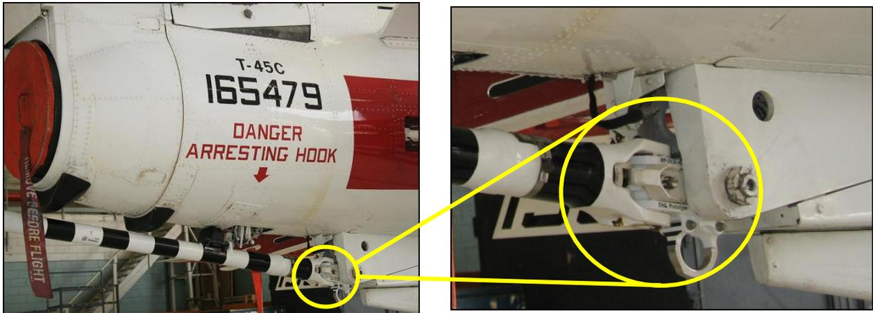
**Figure 6-3. nCoP Plated Pivot Installed on A/C BUNO 165479.**
