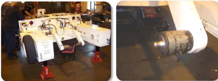
**Figure 4-5. Image of Lifting Arm Pin Installed on Spotting Dolly (left) and Close-up (right).**
