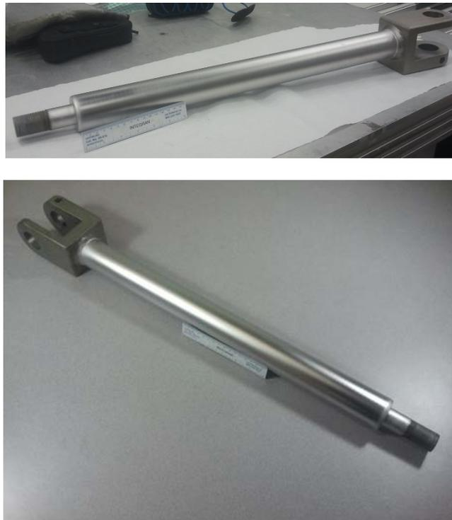
**Figure 6-7. Images of the nCoP Coated component at Integran.**
