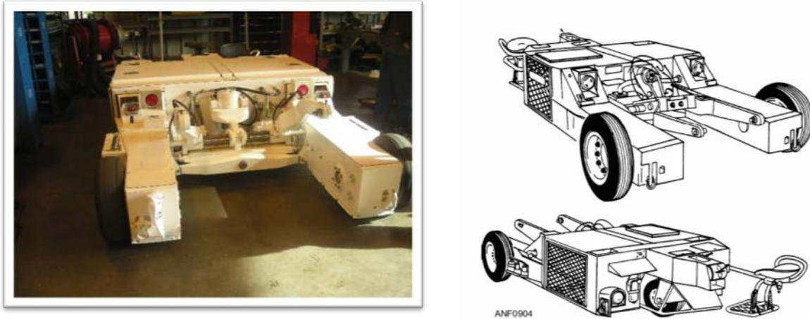
**Figure 4-4. Image of the Spotting Dolly (left) and Schematic Drawing of the Spotting Dolly (right).**
