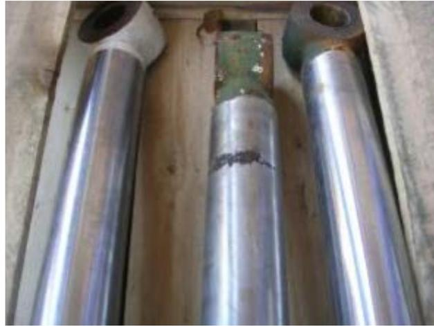
**Figure 4-7. Representative Hydraulic Cylinder Tube Casings from MK48 LVS Disassembled Following Service.**
