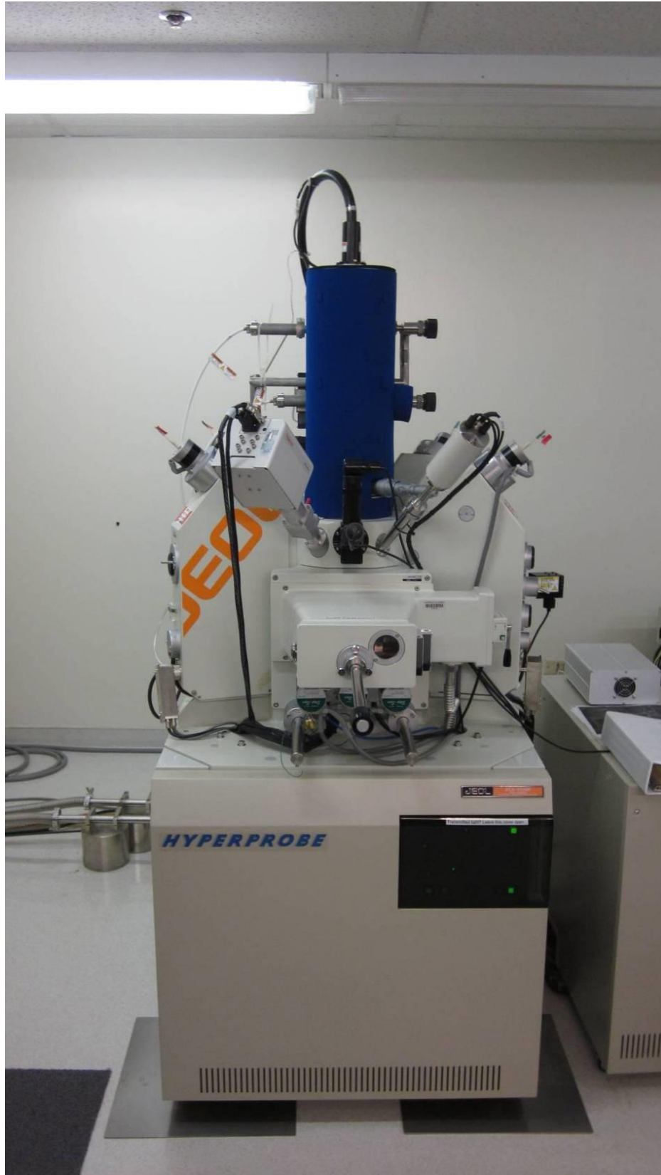
Figure 22. Electron Probe Microanalyzer used in the SEM with EDS analyses
