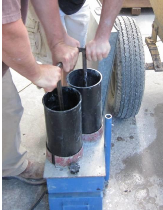
Figure 2. Compaction of the geopolymer cylinders using molds affixed to a shake table
