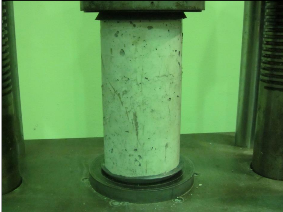
Figure 8. Sulfur compound caps at the ends of a 6-inch-diameter geopolymer. Picture taken prior to testing.
