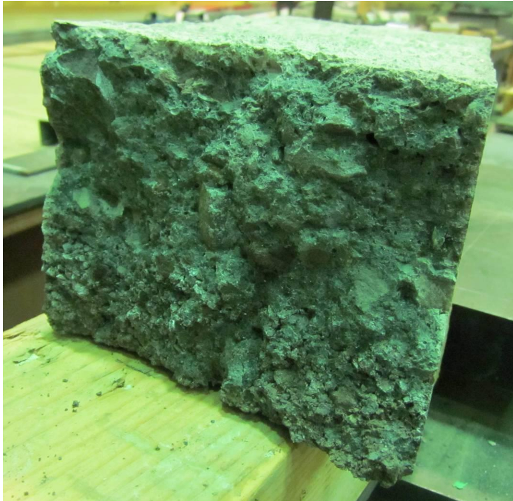
Figure 21. Broken section of a beam after flexure test. Failure occurs mostly between the aggregate and cementitious paste with no shearing through the aggregate observed.
