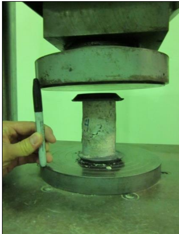
Figure 5. Sulfur compound caps at the ends of a 2.25-inch-diameter geopolymer. Picture taken after testing.
