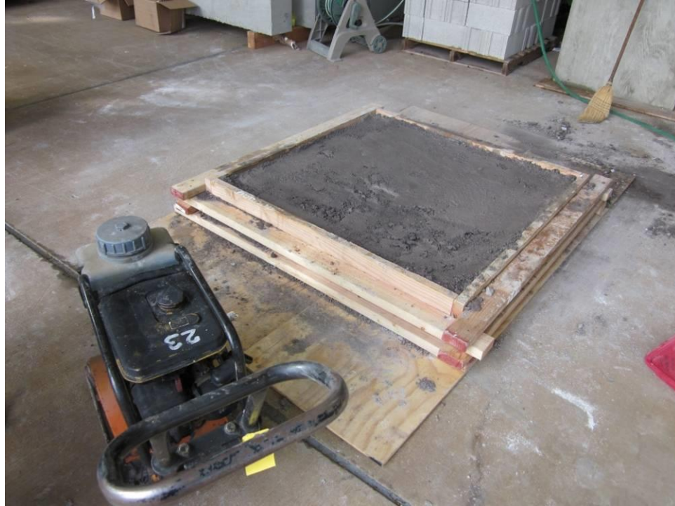
Figure 3. Compaction of the geopolymer slab using a flat plate vibratory compactor
