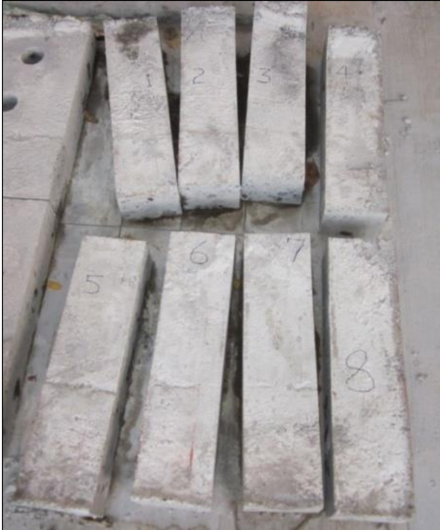
Figure 17. Saw-cut beams used for flexure strength test numbered 1 through 8
