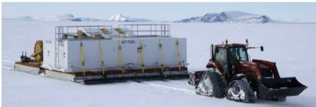
Figure 6. Four ARCS towed outbound on GrIT in 2012. The front pair of ARCS carried two 10,886 kg (24,000 lb) steel tanks. The rear pair carried a 6350 kg (14,000 lb) roller compactor and a tent enclosing tools and spare parts. GrIT12 successfully delivered the tanks and roller compactor to Summit Station on these ARCS.
