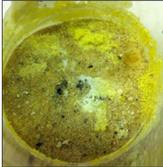
Figure 3. Close-up view of colored DU corrosion products in sand surrounding the fragment of the penetrator rod exposed to salt solution for 14 days (two wet-dry cycles).
