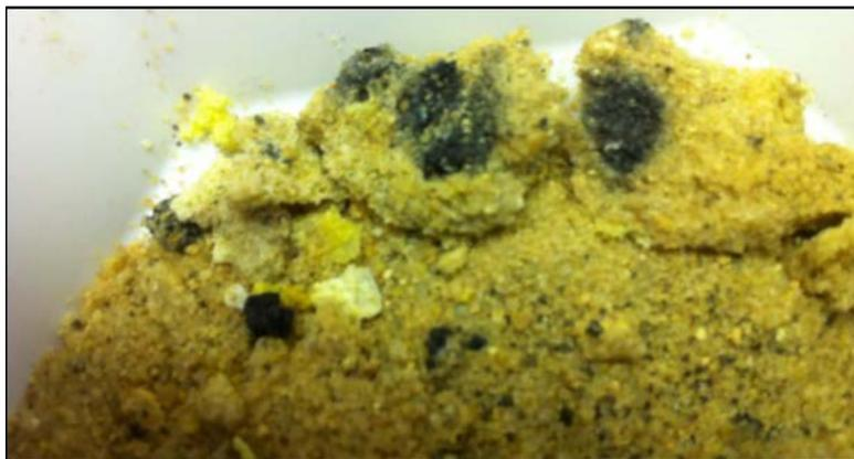
Figure 4 shows fragments containing DU retrieved from the DI water and the salt-solution systems after 28 days of wet-dry cycles. These photo-
