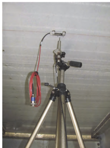
Typical strain gauge and linear varying differential transformer at midspan of fiber-reinforced polymer deck panel.
