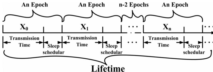
Fig. 3 Network lifetime broken up into epochs<sup>6</sup>
