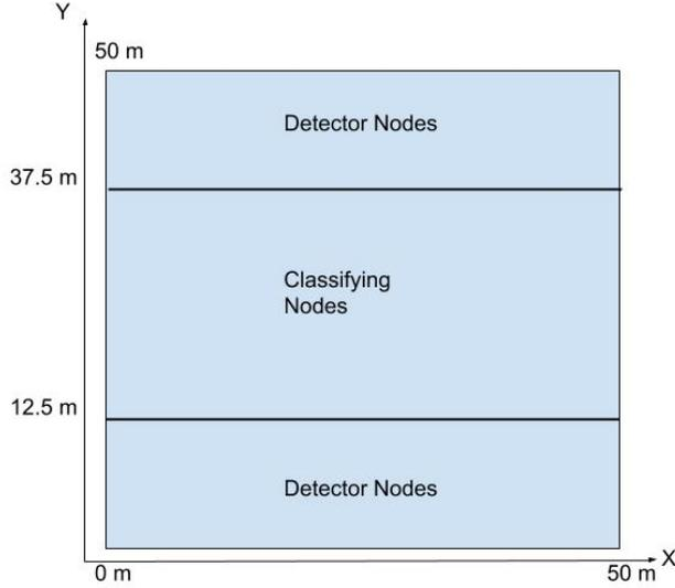
**Fig. 10 Placement of nodes in the network**
