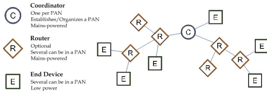
**Fig. 9 Zigbee mesh network layout**
