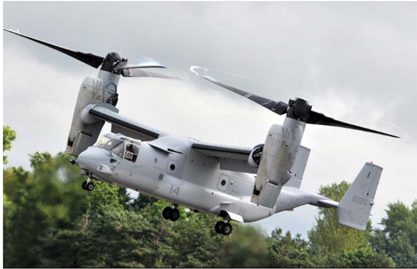
Figure 6. V-22 Osprey taking off vertically, from [7].
