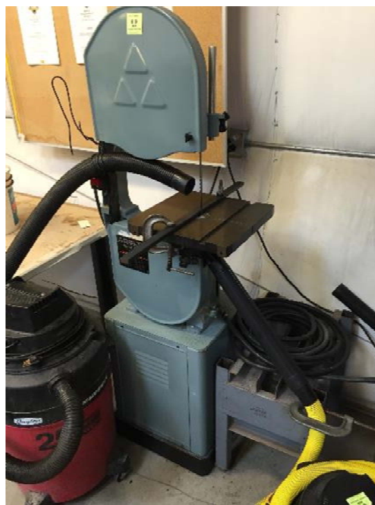
Figure 46. Carbide grit band saw used for trimming fore wing airfoils.
