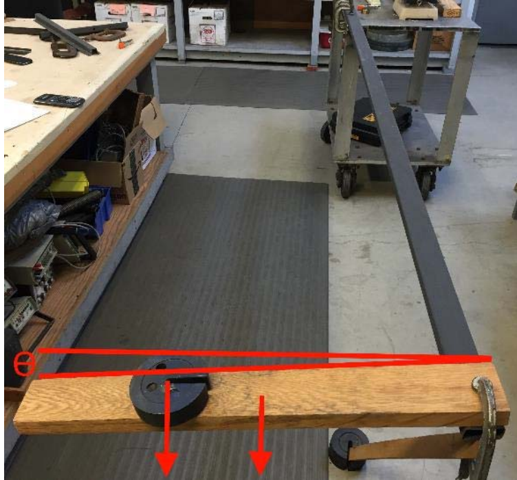
Figure 53. Torsional rigidity measurement experimental setup.
