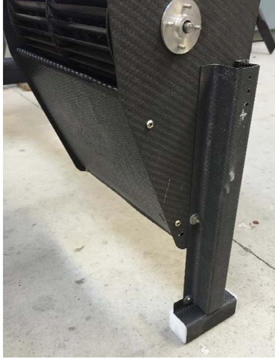
Figure 56. A vertical landing strut.
