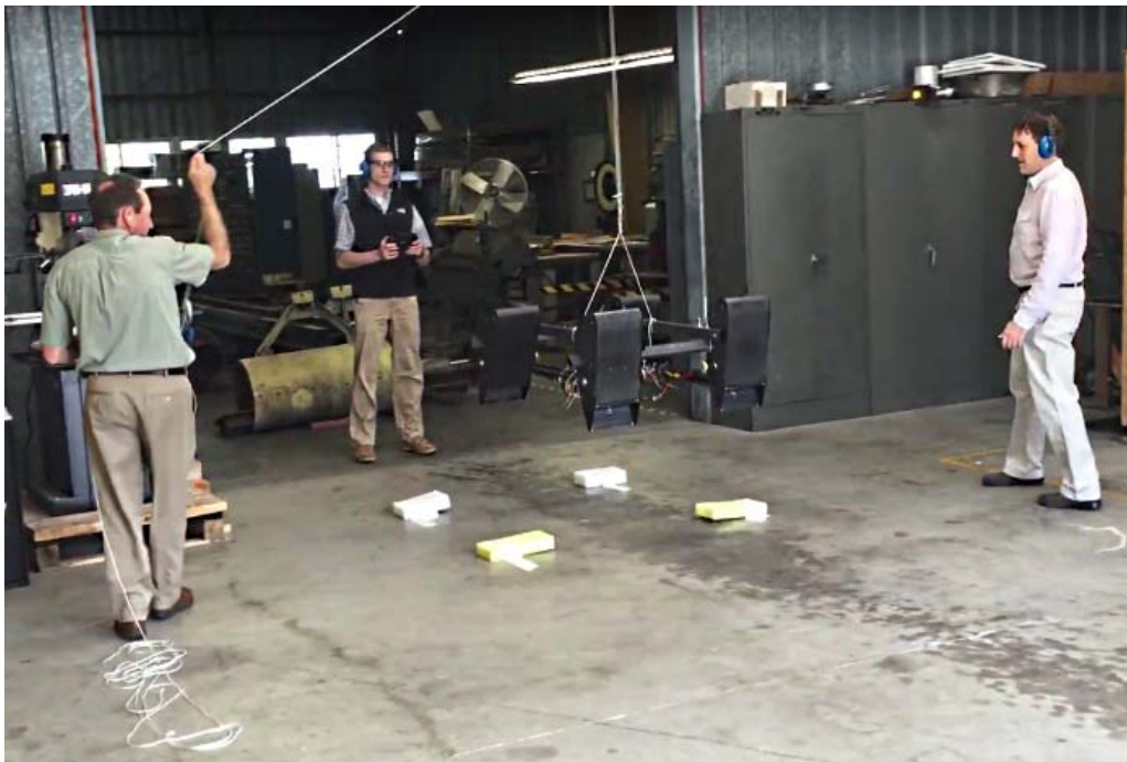
Figure 57. Tethered vertical hover.
