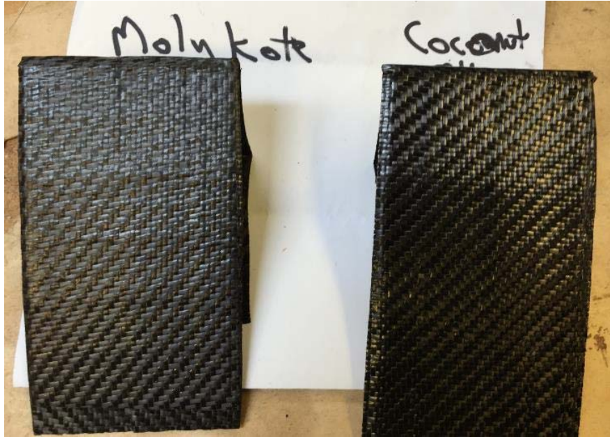
Figure 42. Molykote and coconut oil releasing agent comparison.
