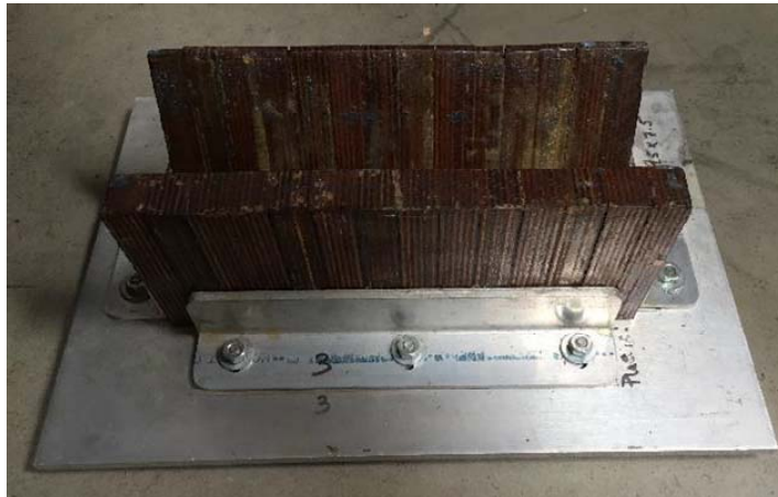
Figure 34. A former wood routed mold used for carbon fiber layup.
