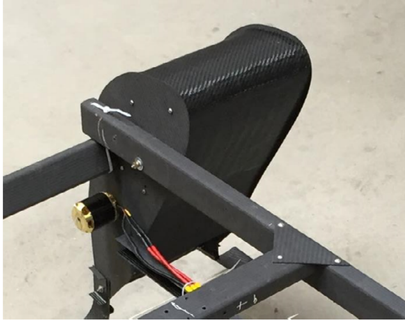
Figure 55. Frame members hooked directly to the endplates.
