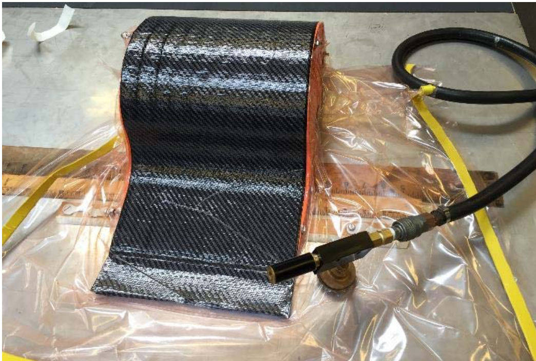
Figure 41. Bagging and vacuum pump usage.
