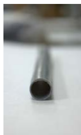
Figure 14 - Cylindrical tube of a ceramic YAG green body, as extruded.
