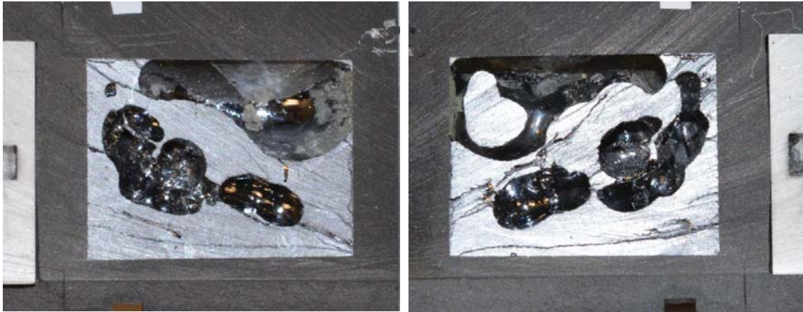
Figure 15: Section Photographs of Graphite Walled Test Section Post Testing
