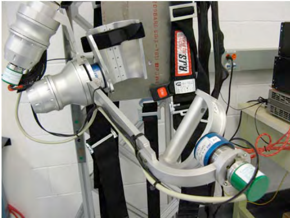
Figure 1: Old upper arm attachment used an elbow brace (left), whereas the new system uses an upper arm brace (right). The JR3 force sensor (blue disc), connects the arm brace to the links.
