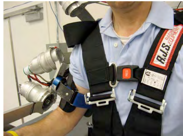
Figure 1: Old upper arm attachment used an elbow brace (left), whereas the new system uses an upper arm brace (right). The JR3 force sensor (blue disc), connects the arm brace to the links.
