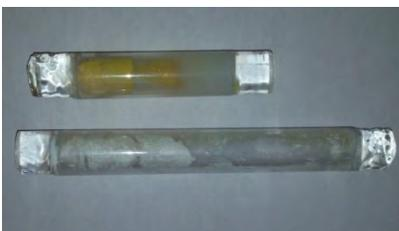
Figure 3.2.1. Erbium doped ZnSe and ZnS powders sealed in quartz ampules.
