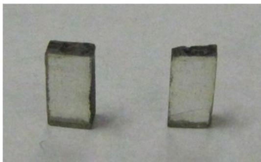
Figure 2.4.10. Fe:ZnS crystals (2×5×7 mm) annealed at 950 °C for 14 days under 44 Rad/s (left) and 0 Rad/s (right).
