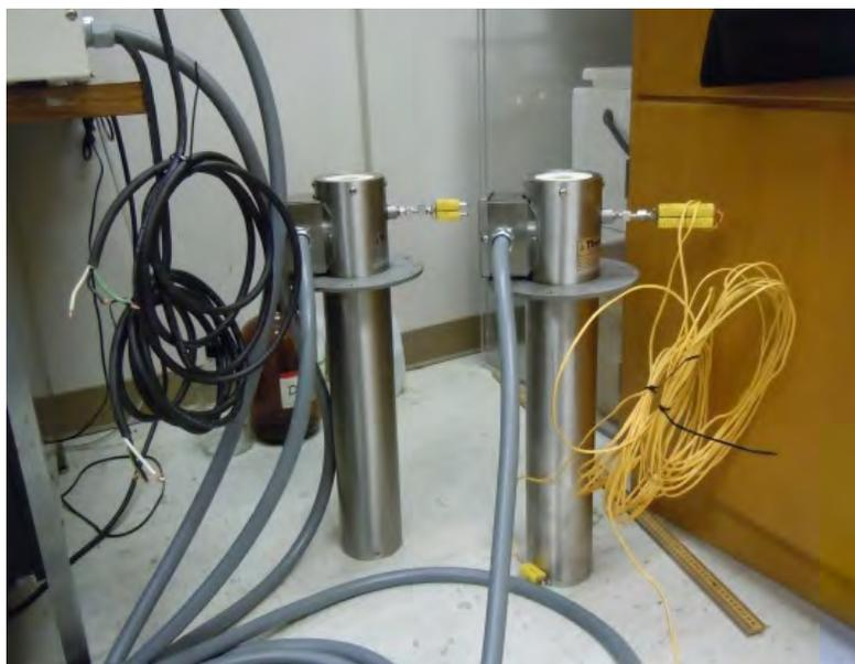
Figure 2.4.3. Two custom made furnaces designed by Thermo Scientific for  $\gamma$ -enhanced thermal diffusion experiments. The furnaces were able to operate long-term under  $\gamma$ -irradiation at temperatures up to  $1000$  °C and accepted up to  $20 \text{ } \phi 9 \times 50$  mm ampoules.
