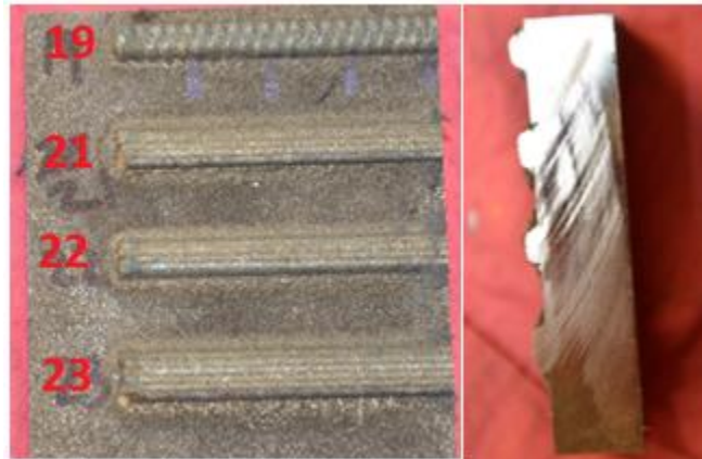
Figure 2: Image of the surface and cross sections of Phase 2 deposition samples.
