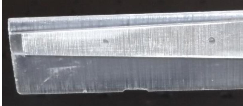
Fig. 5 Photo of canard blade with damaged trailing edge
