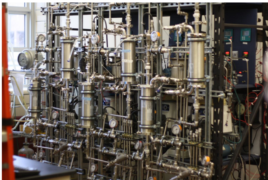
Figure 1: Stainless steel reactor systems designed to examine the effect of hydrogen partial pressures on medium-chain carboxylic acid production. The stainless-steel extraction modules are at the forefront (each bioreactor has two of these modules).
