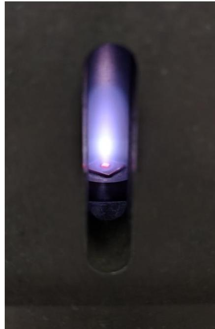
*Growth of superconducting diamond in a highly dense CVD plasma*
