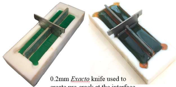
Teflon mold with release holes
