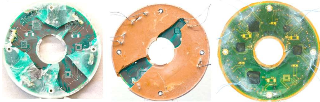
High-g shock tested PCBs at 25,000g
