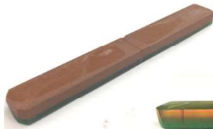
Epoxy-B/PCB cured sample
