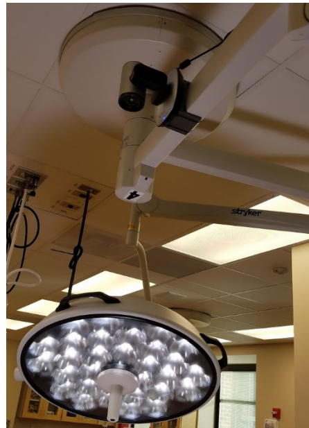
Figure 10. CAD model design and usage of piece to position the top-down camera on the surgical lights mechanical arm.
