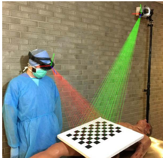
Figure 4: Calibration stage (left): the overhead camera (green ray visualization) is registered with respect to the ARHMD built-in camera (red rays) using a calibration checkerboard. Operation stage (right): The incision line, the scalpel tip, and the textual label stem tip are projected from the overhead camera's perspective onto the surgical field geometry. The incision line lies on the patient, whereas the scalpel and the label annotations float above the patient.
