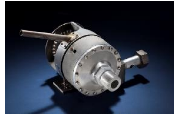
Robert Goddard's First Generation Turbopump
