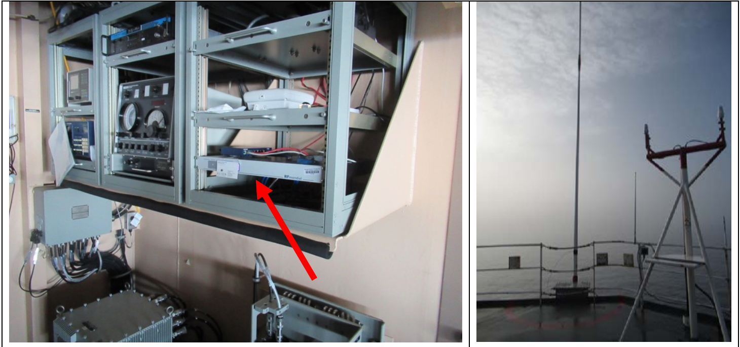
Figure B-13. DRM receiver installed in USCGC HEALY's radio room. The antenna on the port side flying bridge was used.
