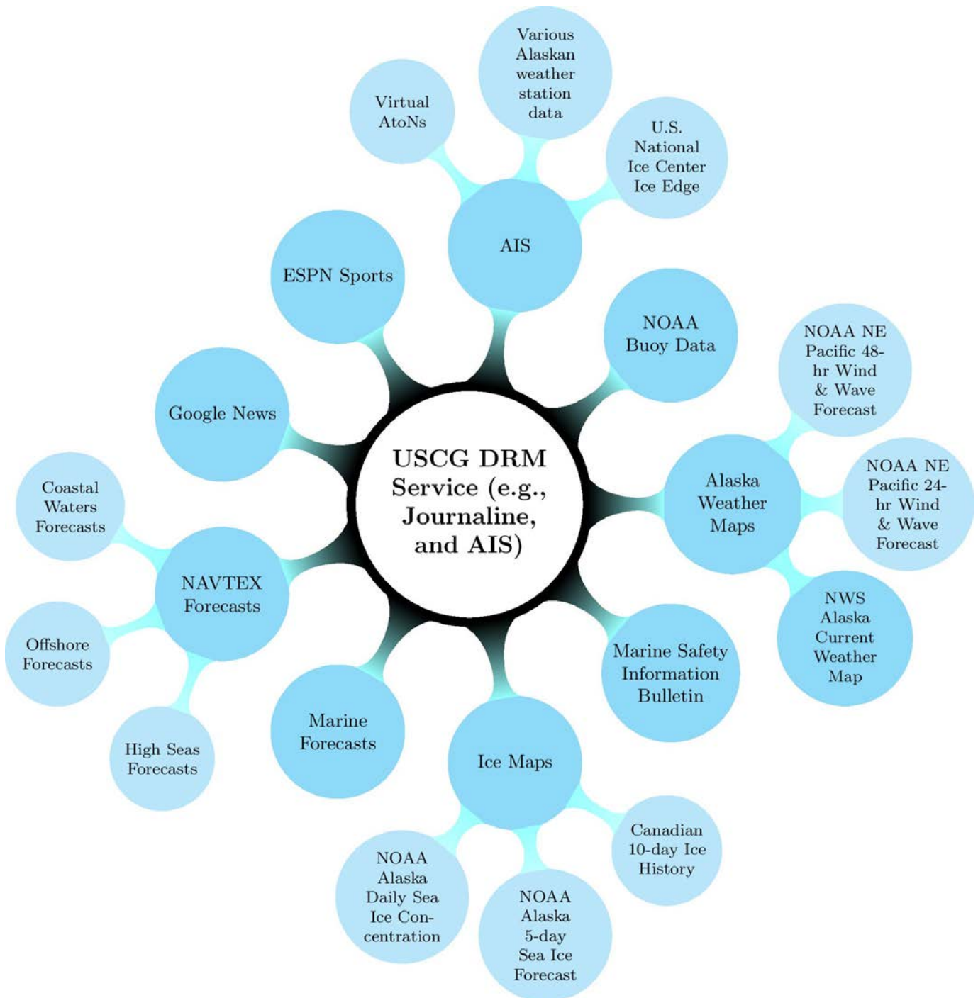
Figure 4. The Fetcher/Formatter software automatically builds the USCG DRM Service feed.
