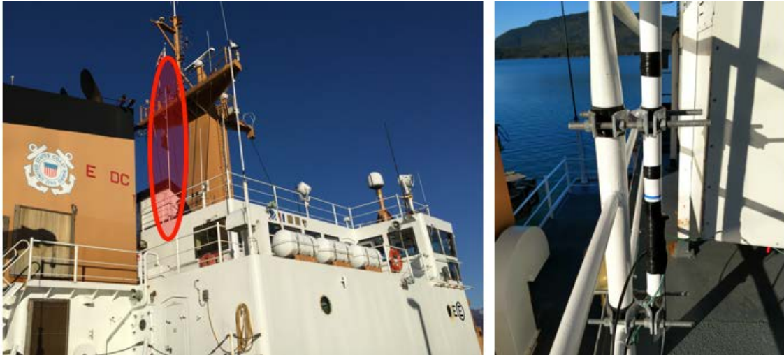
Figure B-11. Antenna (circled in red) mounted to inside of rail on deck above bridge on USCGC SYCAMORE. Close-up of rail mount on right.
