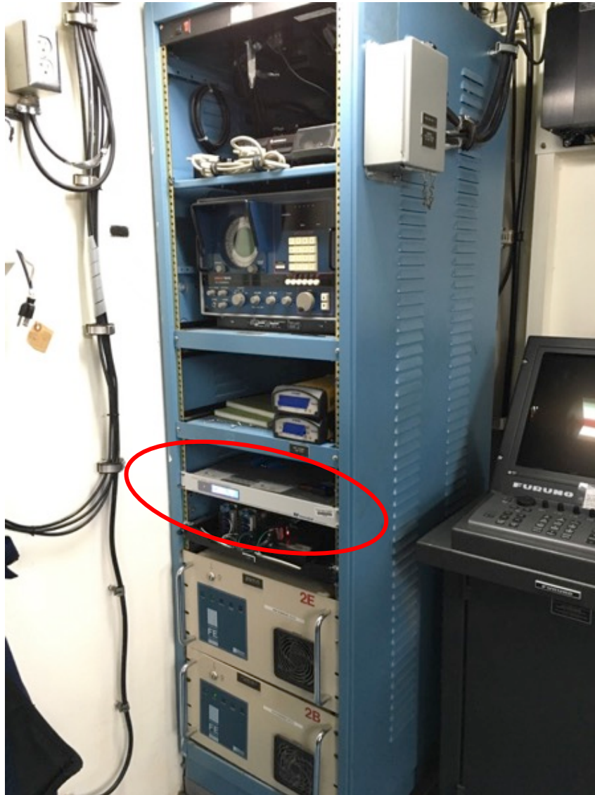
Figure B-10. USCGC SYCAMORE receiver mounted in cabinet rack in bridge chart room.
