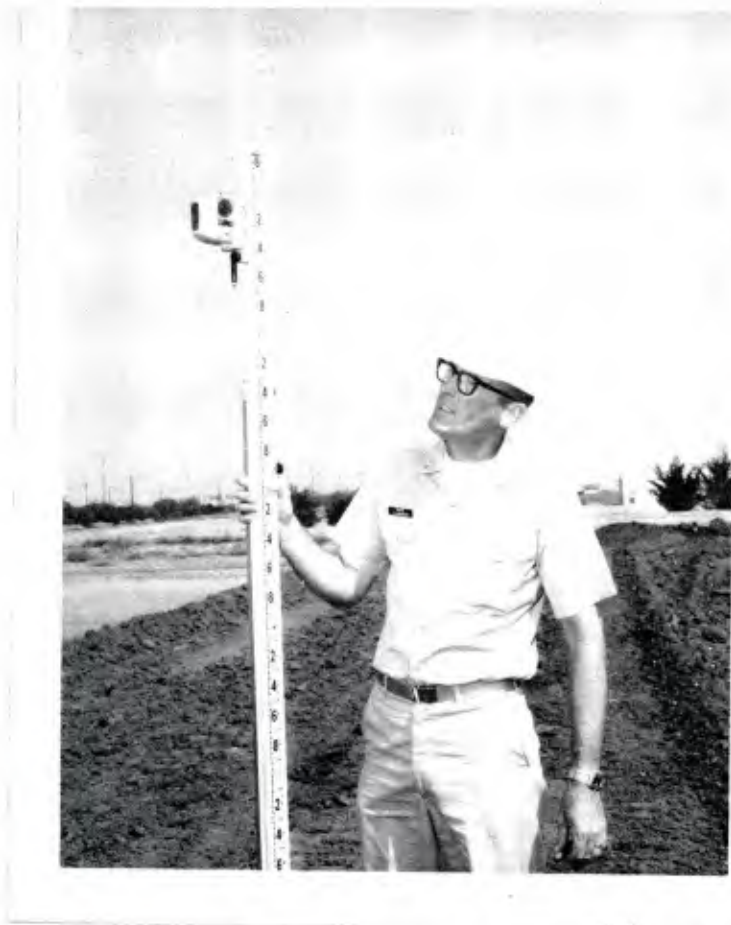
Figure 1. Surveyor's rod of Laserplane surveying system. Using the photocell detector and Lenker tape, one man can obtain elevation readings with this type of system.
