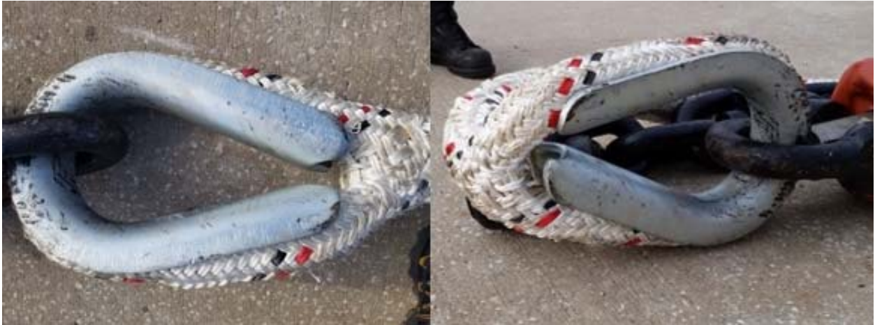
Figure 17. Mooring rope eye splices and thimbles.
