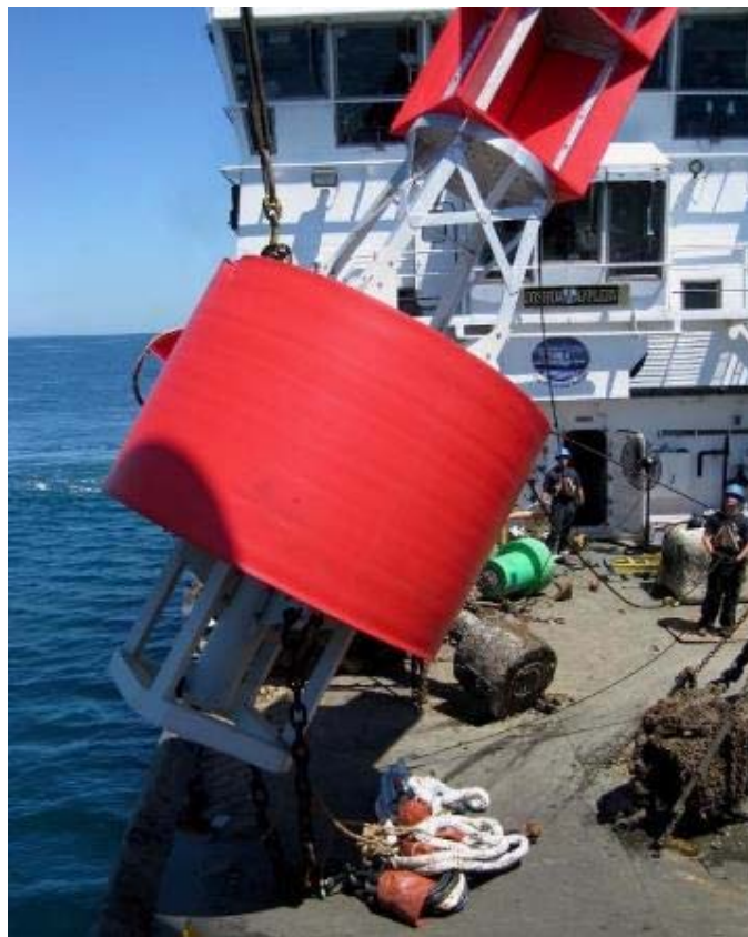
Figure 42. Superflex EFBMS attached to 8X22LFR Egmont Channel R "6" before deployment.
