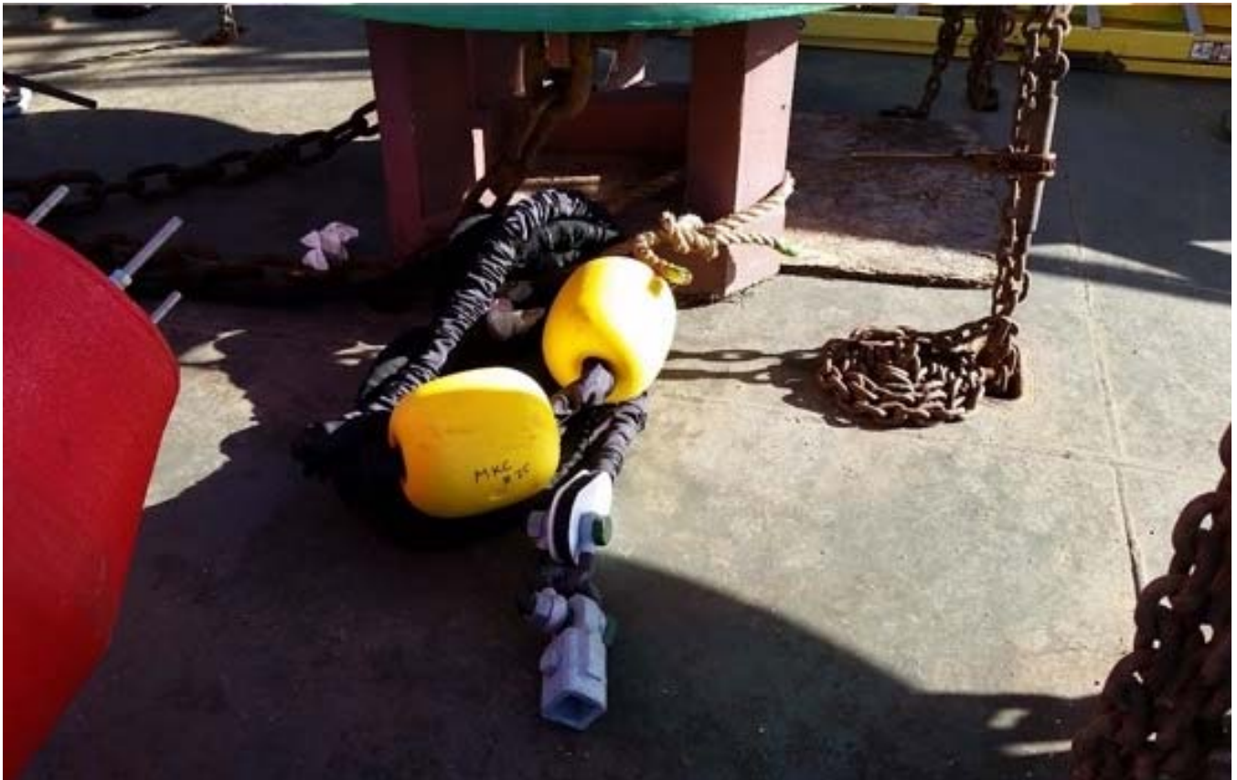
Figure 25. StormSoft mooring system #3 connected to buoy on buoy deck with helix anchor mooring termination head.
