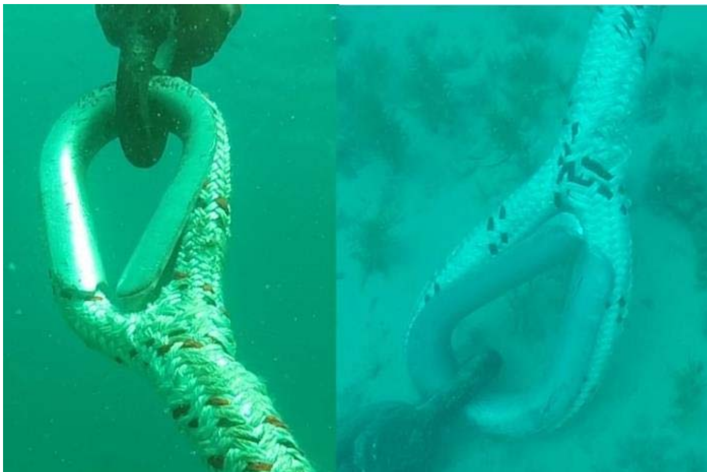
Figure 47. Superflex EFBMS mooring rope loose eye splices around thimbles.
