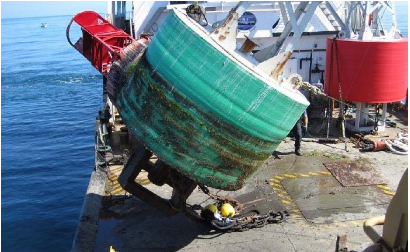
Figure 39. Egmont Channel G "5" with nine feet of 1.5-inch chain connecting the StormSoft EFBMS with the bridle.
