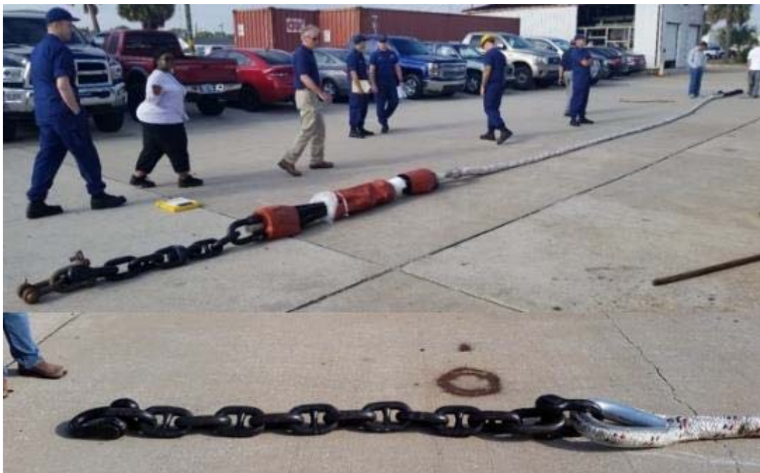
Figure 16. Superflex SB18020 mooring system ends.
