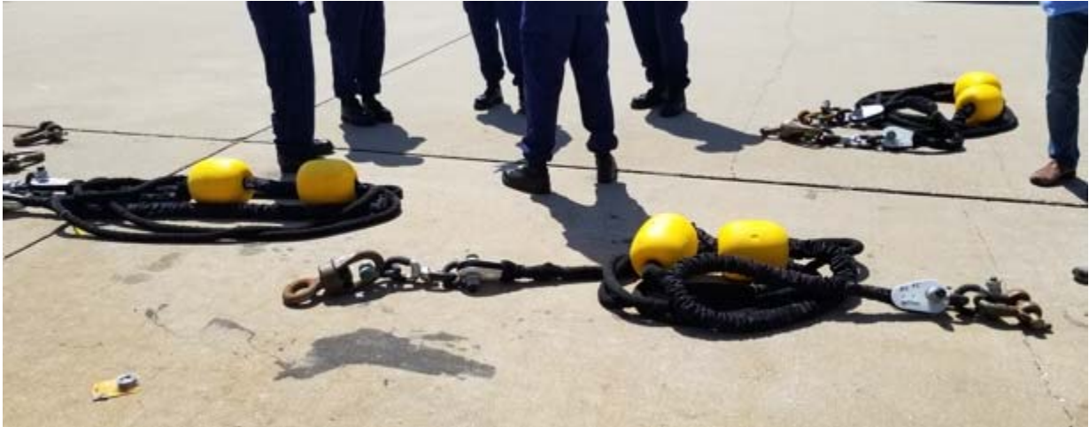
Figure 21. StormSoft mooring lines.
