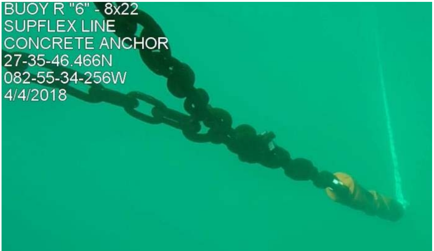
Figure 45. Superflex EFBMS SB18020 shock absorber and buoy bridle.
