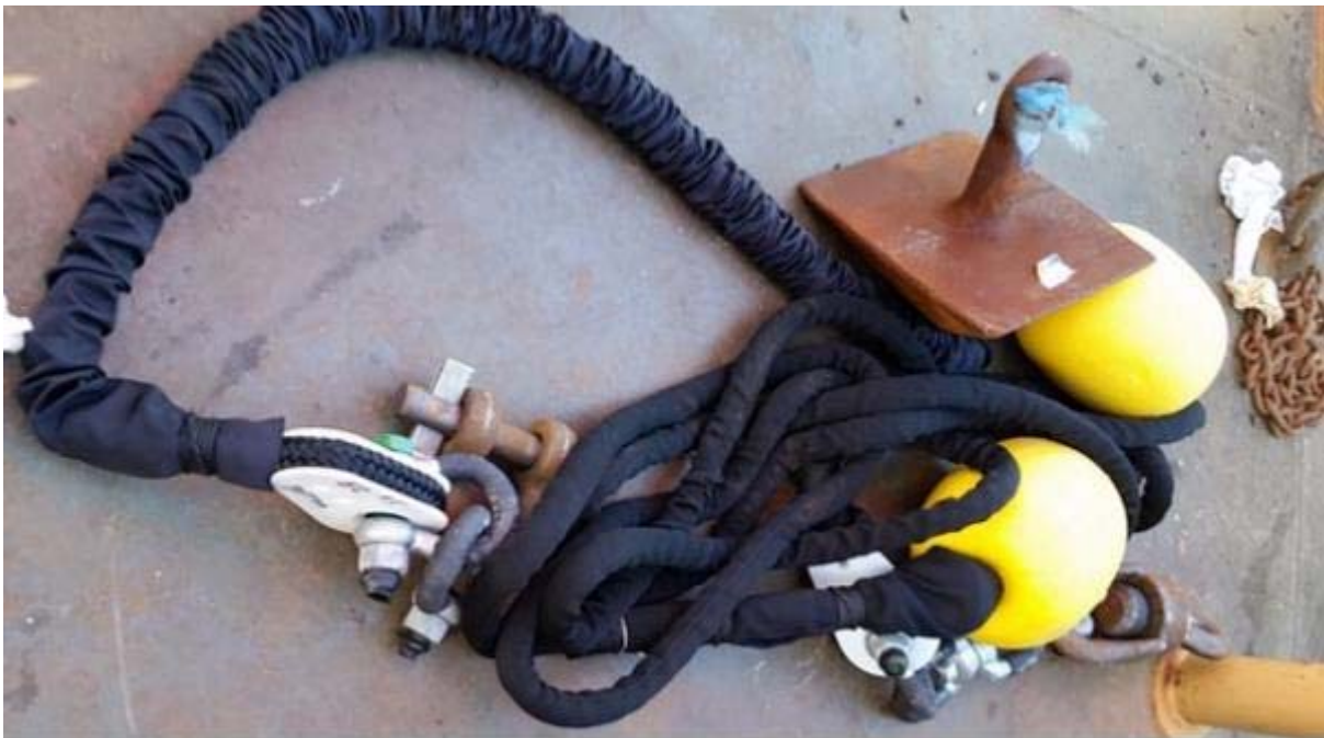
Figure 23. StormSoft mooring system #1 on buoy deck.
