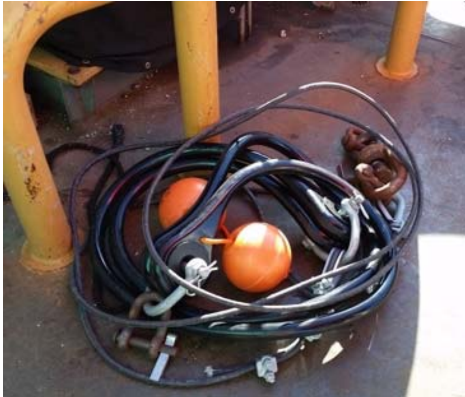
Figure 27. Hazelett Marine mooring system on buoy deck.
