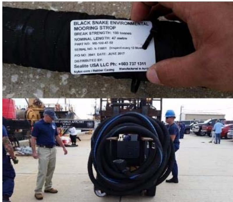
Figure 19. Sealite mooring line.
