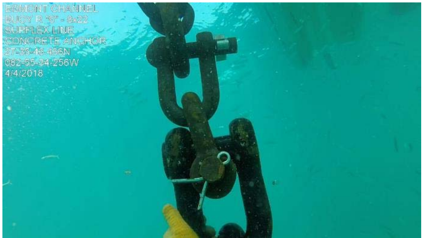
Figure 44. Superflex EFBMS connection to 2 nd Class swivel, shackle and chain.
