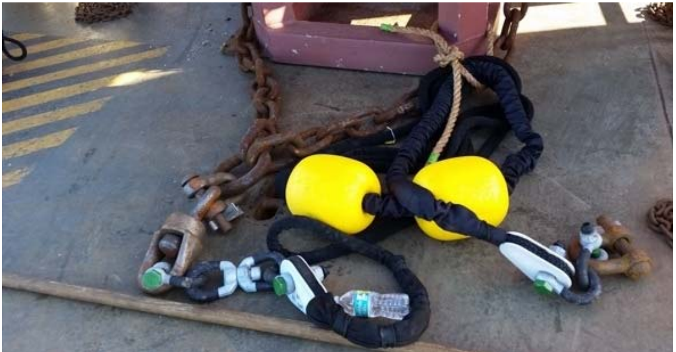
Figure 24. StormSoft mooring system #2 connected to buoy on buoy deck with CG swivel and shackles.
