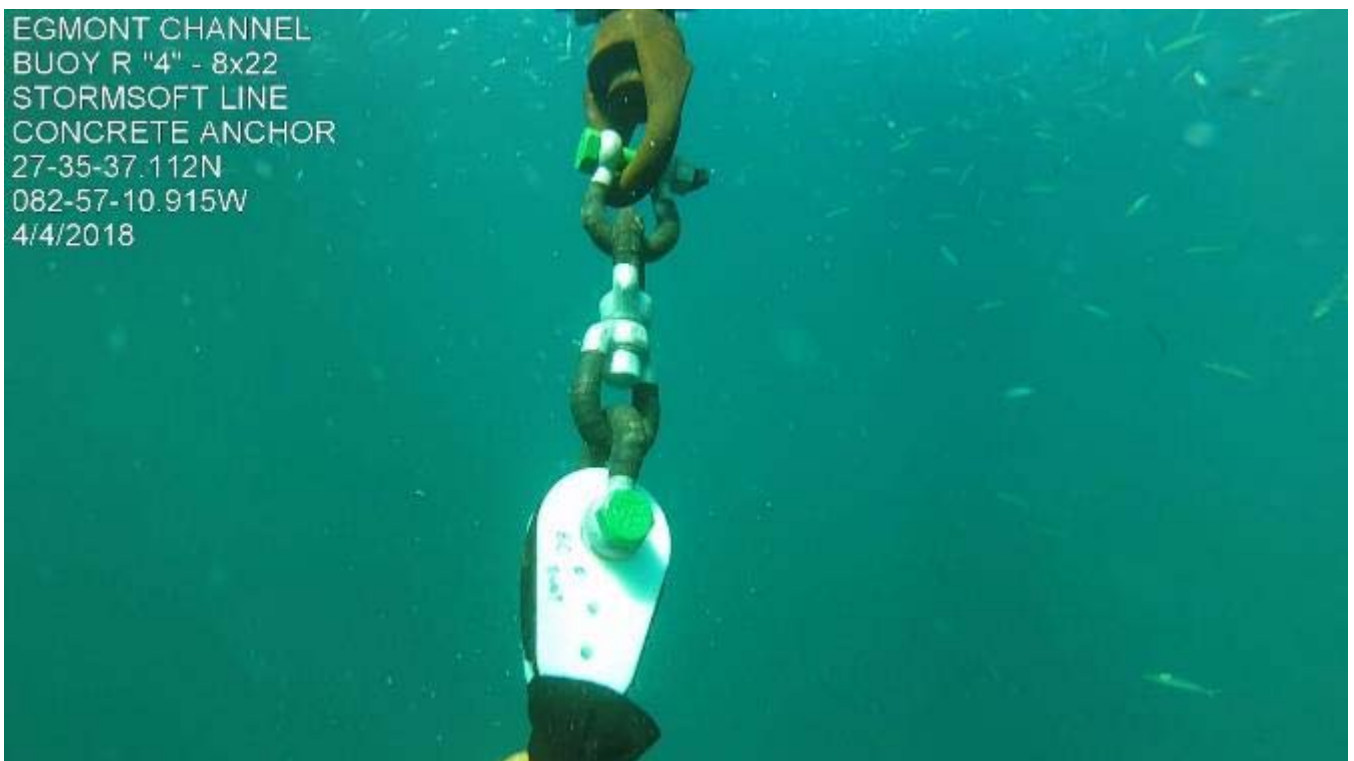
Figure 38. StormSoft EFBMS connection to CG 3rd Class swivel at buoy bridle.
