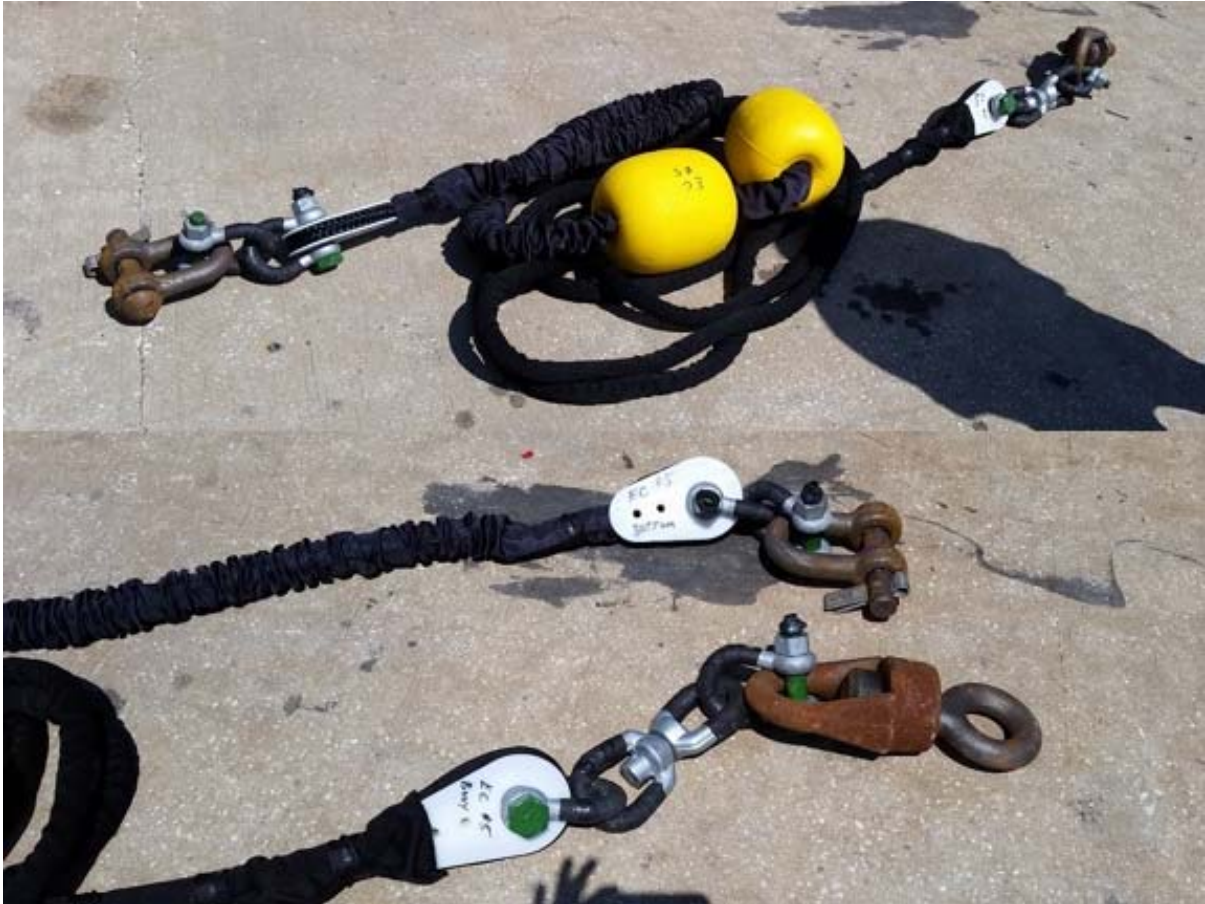
Figure 22. StormSoft mooring system #1 with CG swivel and shackle.
