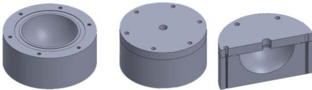
Figure 32. Proof-of-concept die for superplastic formation studies
