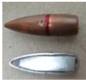
Figure 1. Cutaway of 7.62x39mm ball round
