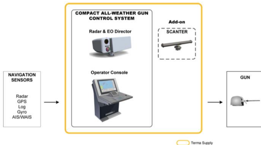
Figure 8. COMPACT All Weather Gun Control System. Source: Terma (2012f).
