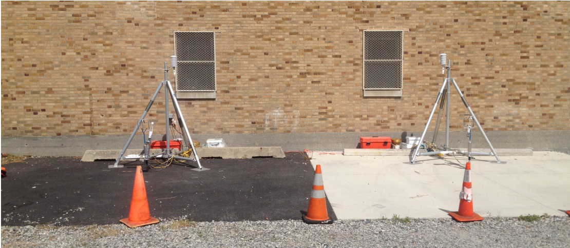
Figure 1: Flux towers installed at Manhattan College. Left: Asphalt. Right: Concrete.
